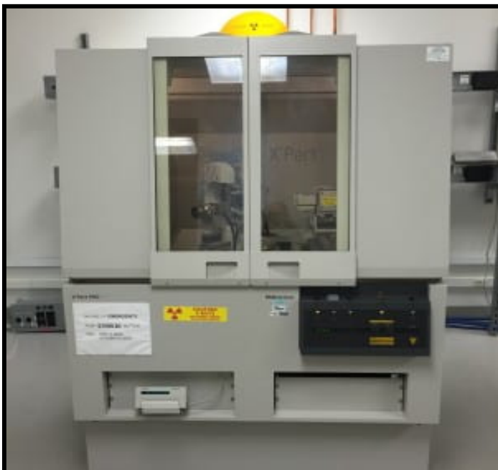
Fig. 4: Picture of XRD machine used for the XRD analysis
