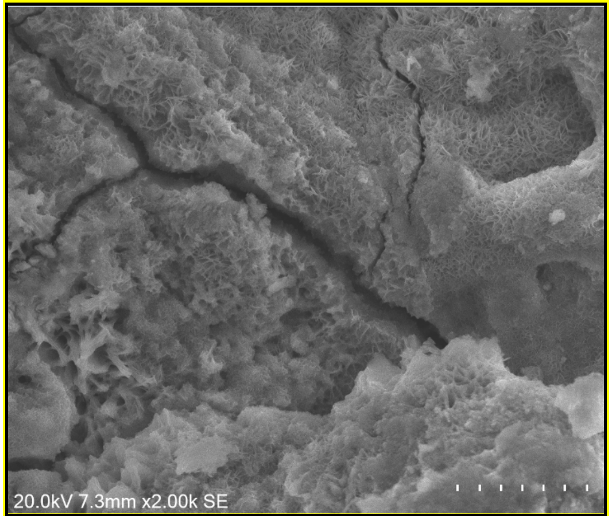
Fig. 39: SEM image of the heat-treated sample at 910 °C after corrosion test with 2000x magnification
