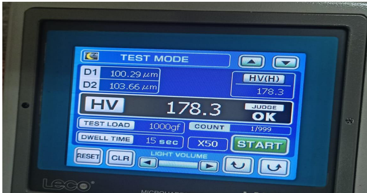
VICKER'S micro hardness test result of tata tiscontmt bar
