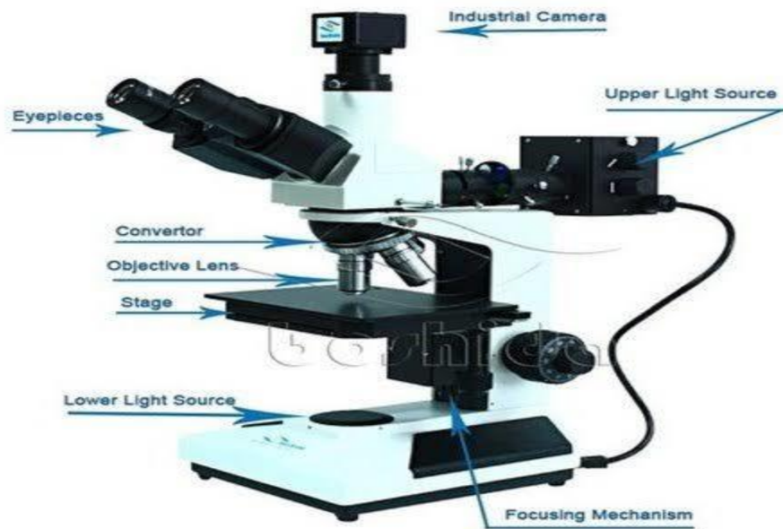
Figure 12: different parts of optical microscope
