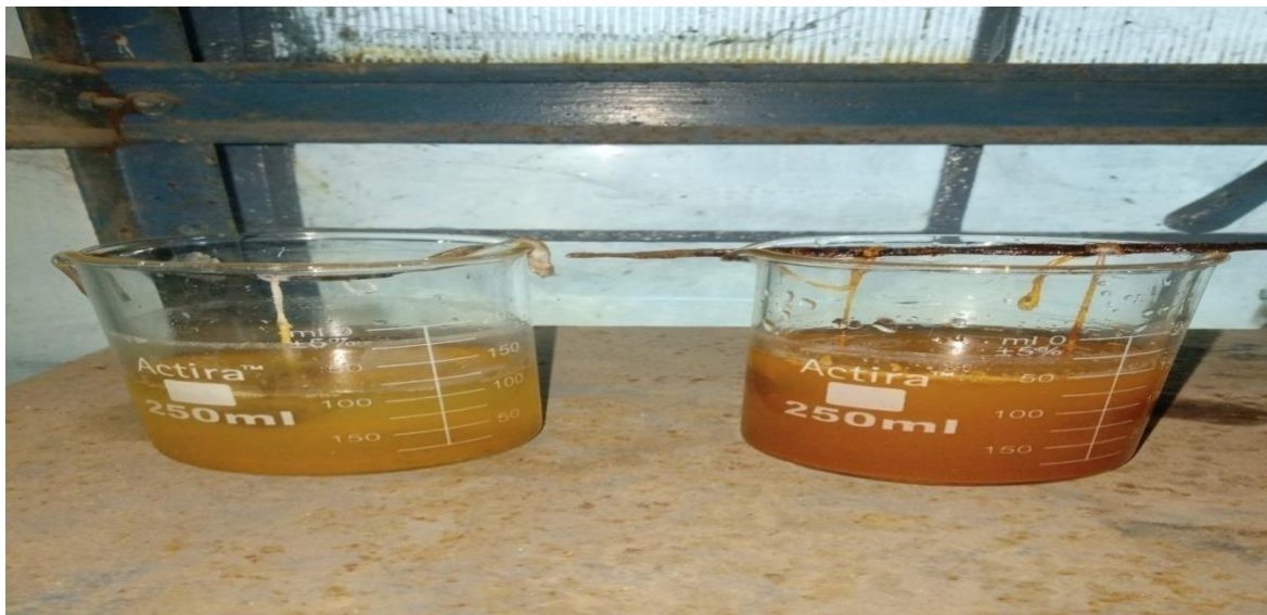
Figure36:corrosion of tmt bars
