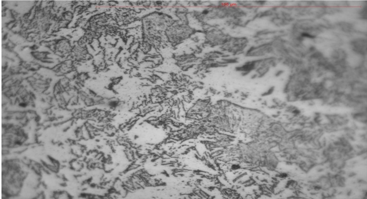
Figure17:microstructure of as received srmbtmt rebar with 1000x resolution
