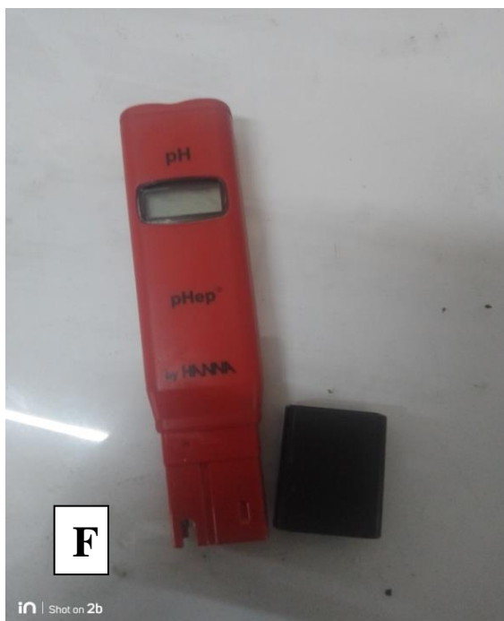
Fig 3.1 Various tools and apparatus for making the required solutions. A. Double Distillation setup B. Weighing scale C. Thermometer D. Conical Flasks E. Beakers F. pH meter
