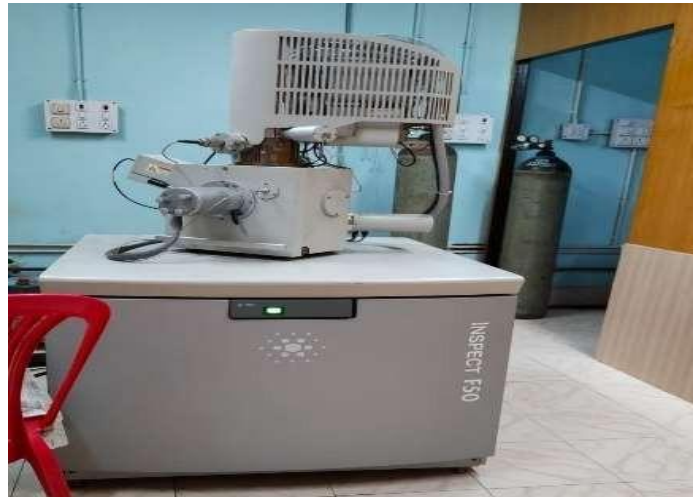
Figure 10: FESEM and EDS measuring instrument
