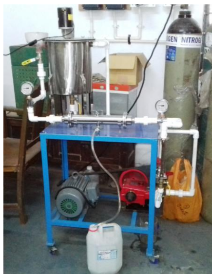
Figure 3: Membrane filtration Pump Setup
