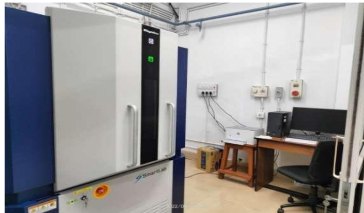
Figure 9: SmartLab SE XRD measuring instrument
