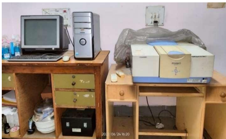
Figure 8: IR Prestige-21 FTIR measuring instrument
