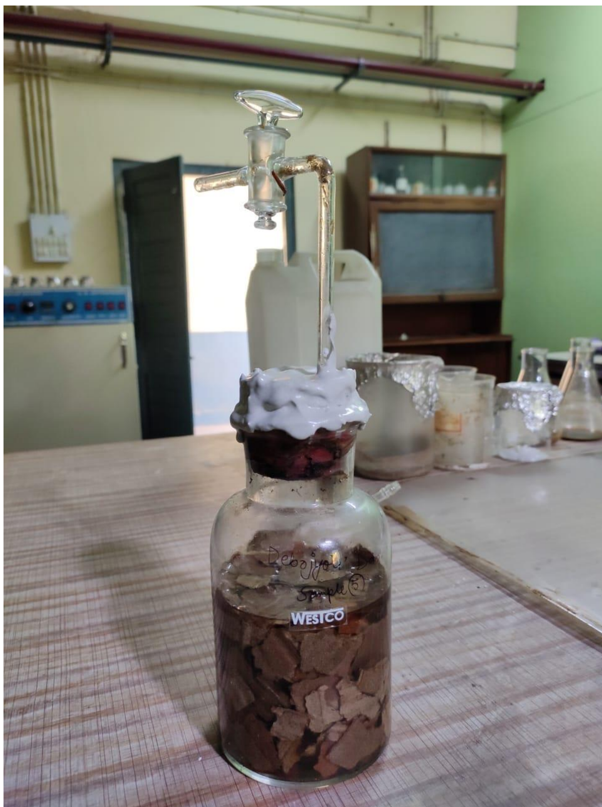
Fig 4.2: 500 ml digester containing only paper waste and water (PW)
