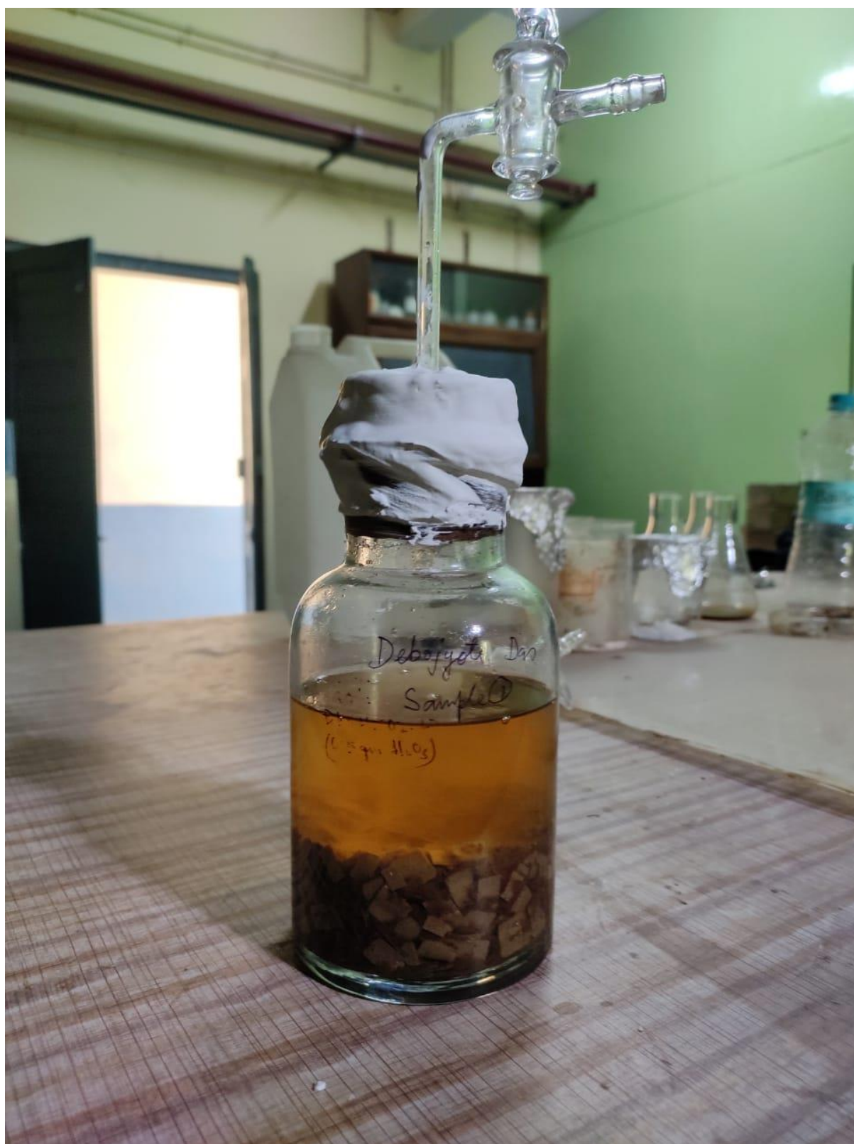
Fig 4.3: 500 ml digester containing paper waste and cowdung in 1:1 ratio (PW:CD)
