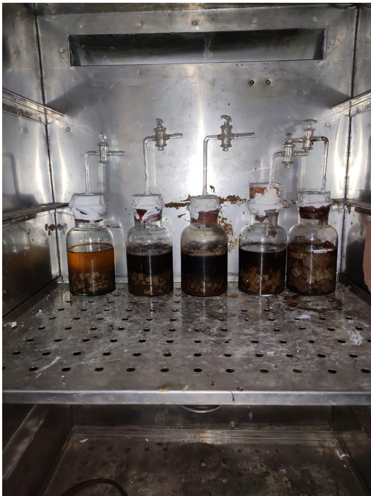
Fig 4.4: Digesters kept inside the incubator at 37 °C
