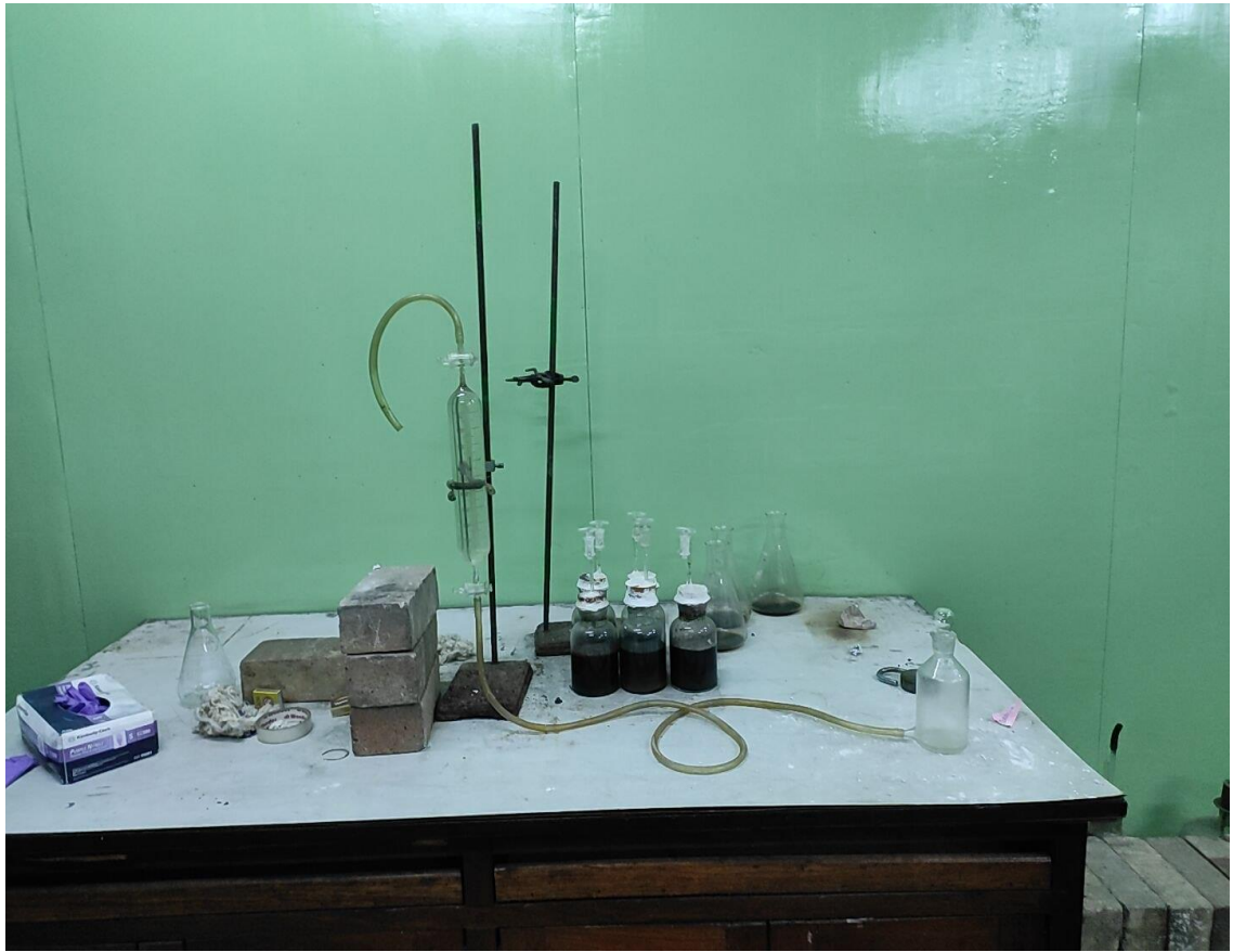
Figure 3.4: Apparatus to measure Biogas by downward displacement of water
