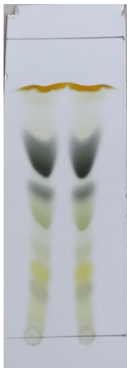
Figure 9: Illustrating distribution of compounds of different polarities after separation on a TLC plate
