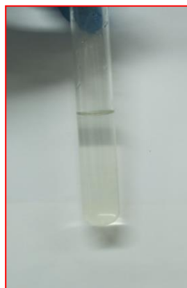
1 ml sample + 2ml 2% NaOH + few drops of dilute HCL (5-7 drops) fig-5.0
