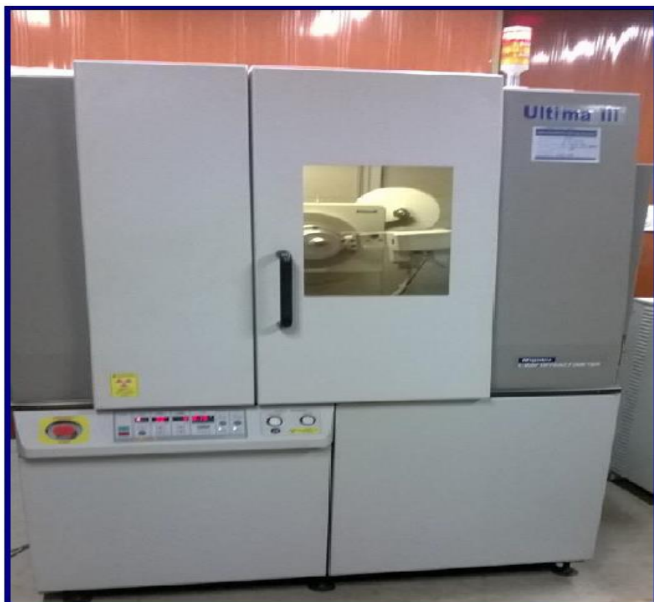
Fig 3.4- Experimental set up of X-Ray Diffractometer.
