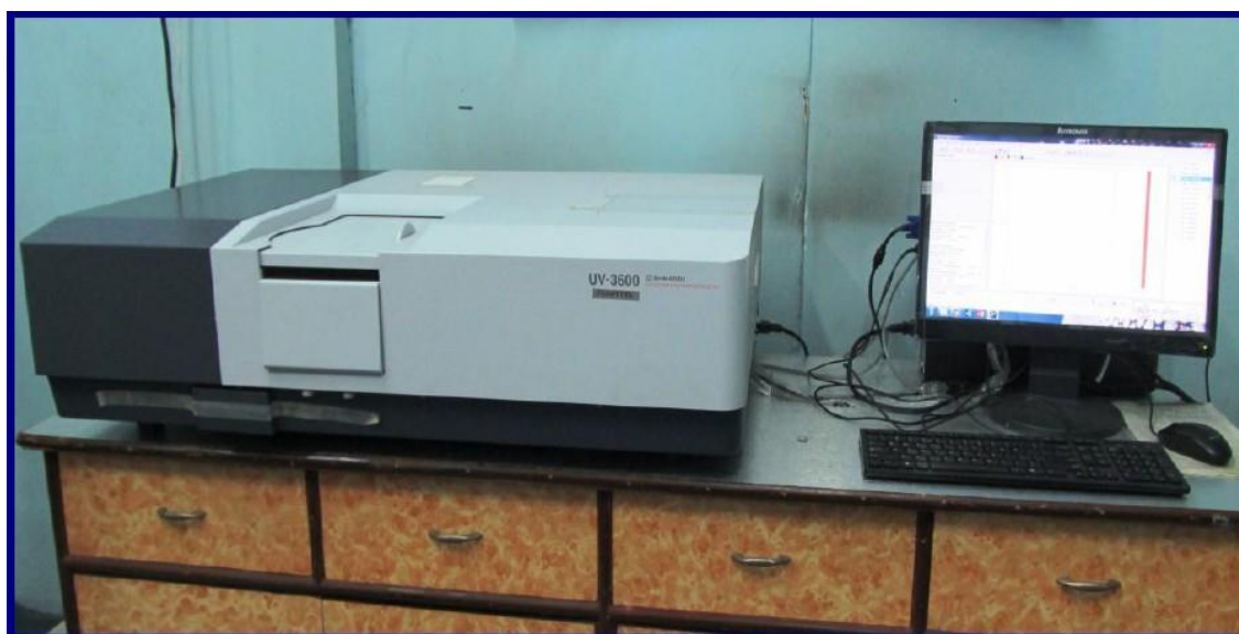
Fig 3.8- Experimental set up of UV-Visible spectrophotometer.
