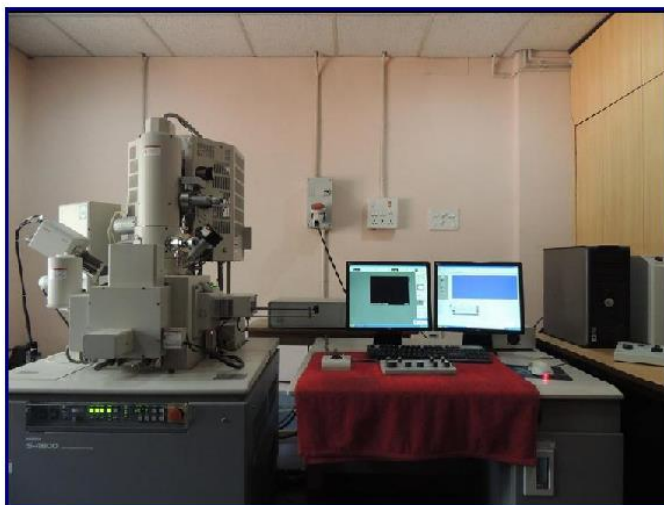
Fig 3.11: FESEM (Hitachi S-4800) set up.
