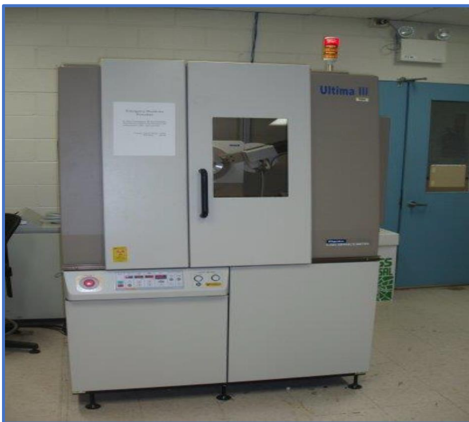
Figure 3.8: Experimental set up of X-Ray Diffractometer
