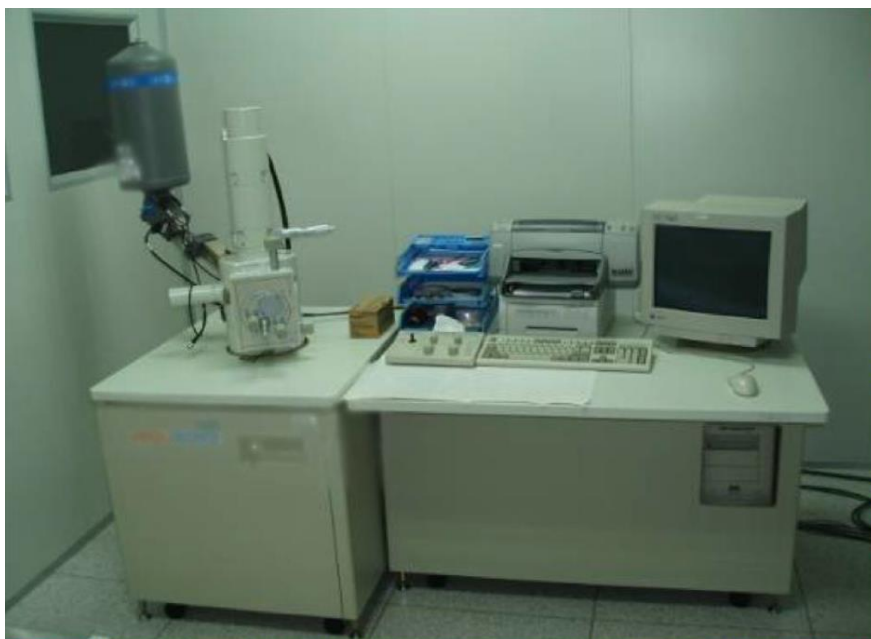
Fig 3.15: Experimental set up of Energy dispersive analysis of X-rays (EDAX).
