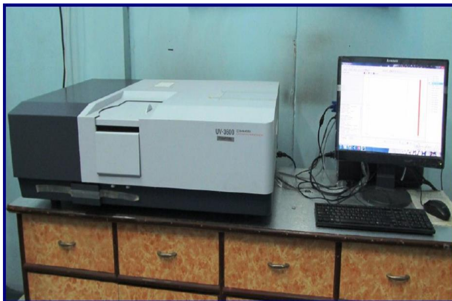
Fig 3.14: Experimental set up of UV-Visible spectrophotometer.
