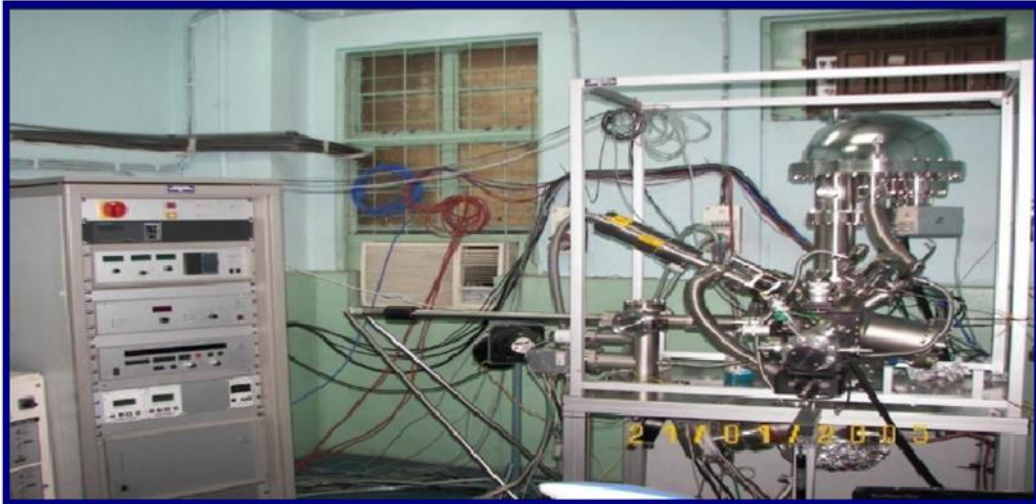
Fig 3.18: Experimental set up of XPS
