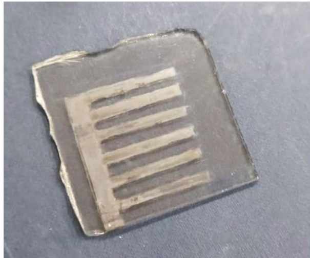
Fig 6.2. Digital photograph of one-sided support and detective electrodes
