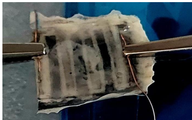
Fig 6.5. Digital Picture of final rGO based flexible symmetric CI supercapacitor.
