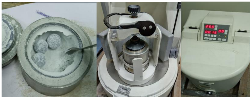
Figure 3.1 PULVERISETTE 6, FRITSCH, Germany, planetary monomill system.
