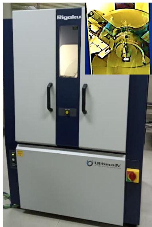
Figure 3.3 Rigaku Ultima IV, multipurpose X-Ray Diffraction system; inside view (inset)
