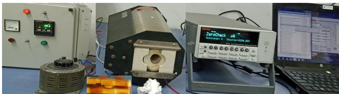
Figure 3.4 Keithley 6517B Electrometer/ High Resistance Meter and Furnace system (0.48kW).
