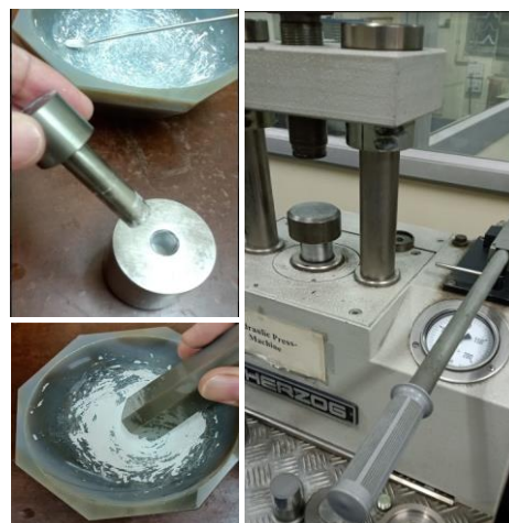
Figure 3.2 Pellet mold set with mortar and pestle; and the hydraulic press used in this study.
