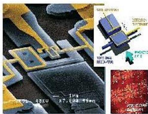
Fig.1.5 A nanometer scale mechanical electrometer consisting of following things a torsional mechanical resonator, a detection electrode, and a gate electrode used to couple charge to the mechanical element[30].
