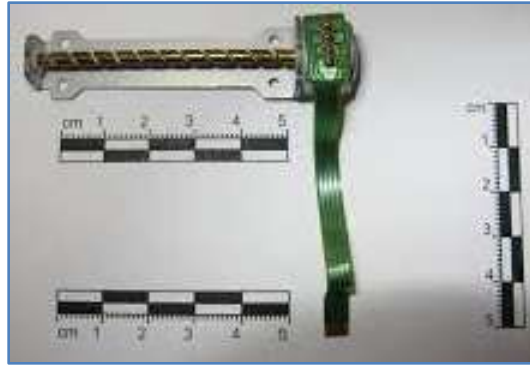
Fig.4.12.(h)Motor lead screw (40cm x 40cm maximum working area)
