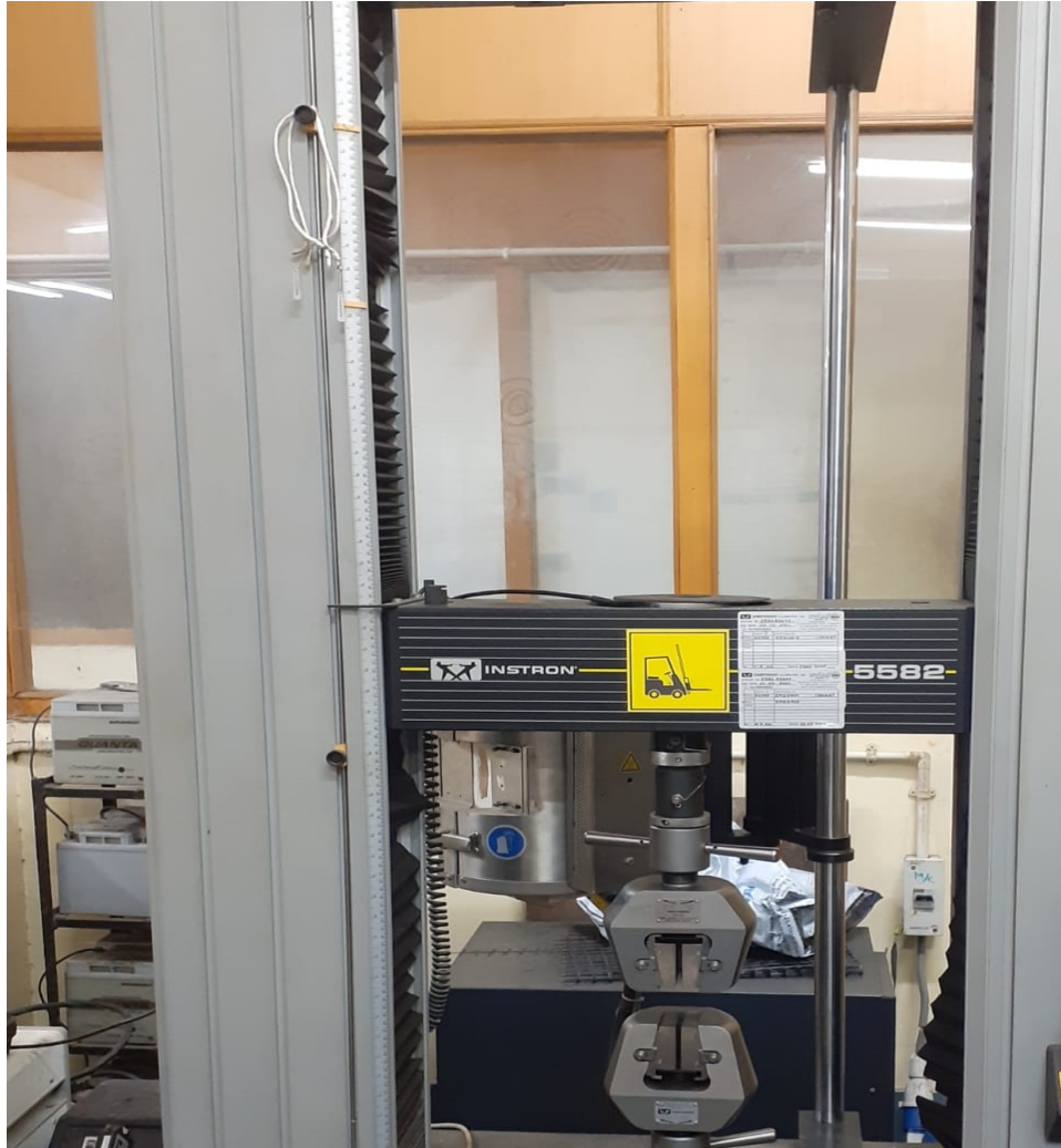
Fig. 3.4 Instron 5582 tensile testing machine
