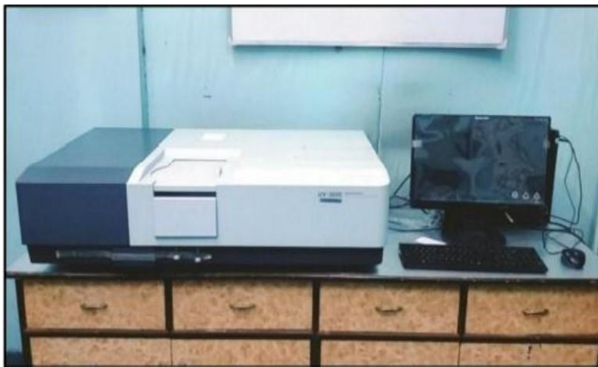
Fig 4.8: Experimental set up of UV-VIS-NIS (SHIMADZU UV-3600) Spectrophotometer
