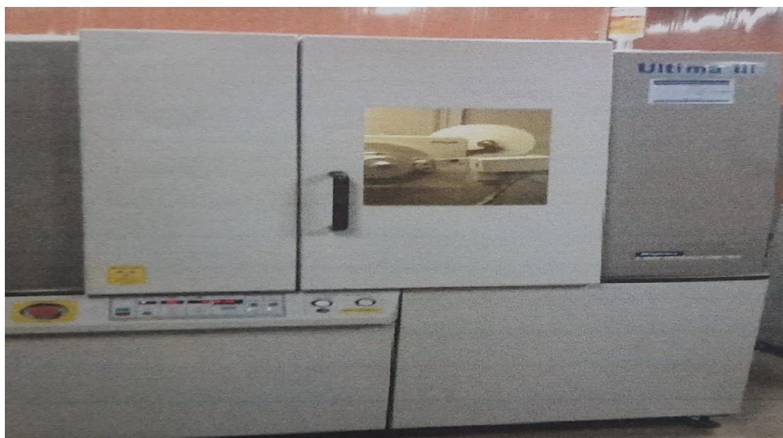
Fig 4.4: Experimental set up of X-Ray Diffractometer
