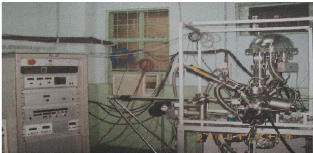
Fig. 4.15: Experimental set up of XPS
