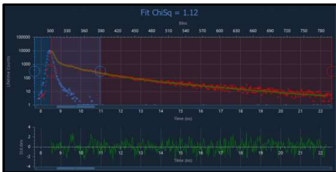
Figure – 5: Fluorescence decay of the dyad –clp system in ACN-sucrose solution, \text{ex} = 375 \text{ nm} , \text{em} = 480 \text{ nm} , the fast (blue) decaying component represents impulse response (diode laser) ( \chi^2 \sim 1.12 ). The residual is also shown.
