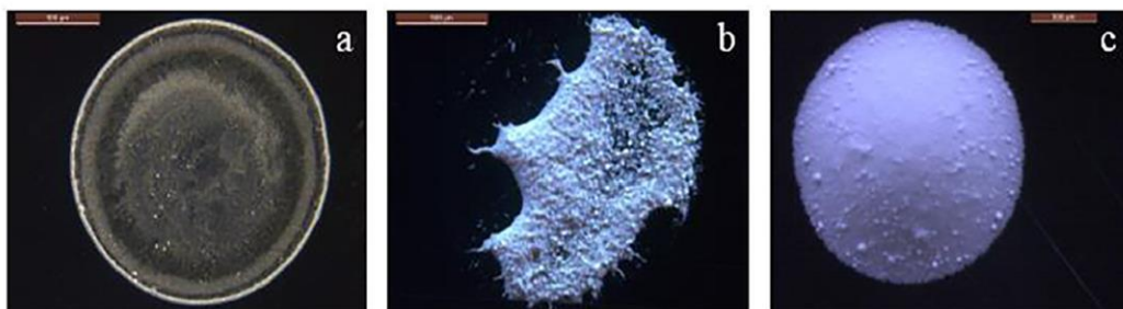
Fig. 1.3h: Comparison of the residue patterns of \text{Al}_2\text{O}_3 nanofluids in different particle sizes and concentrations (a) 9 nm 0.01 vol%, (b) 80 nm 0.5 vol% and (c) 135 nm 4 vol% on stainless steel. The scale bar is 500 \mu\text{m} .
