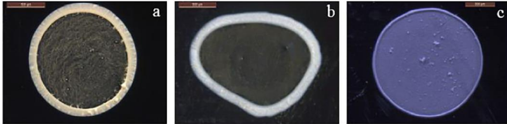
Fig. 7. Comparison of the residue patterns of 0.1 vol% \text{Al}_2\text{O}_3 nanofluid of different particle sizes (a) 9 nm, (b) 13 nm and (c) 135 nm on stainless steel. The scale bar is 500 \mu m.
