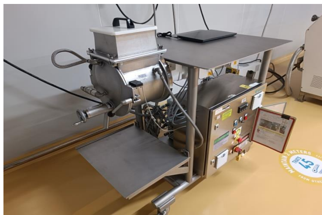
Fig.1.1.3: Elk Conche of capacity 5kg
