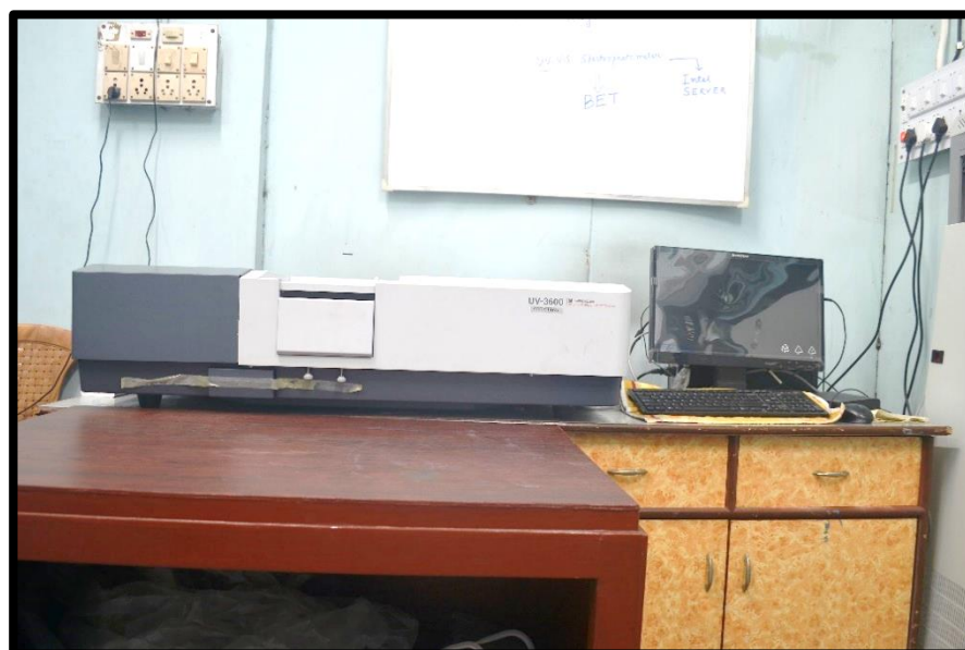
Figure 3.10: Photograph of Shimadzu UV-Vis-NIR (UV-3101-PC) spectrophotometer.
