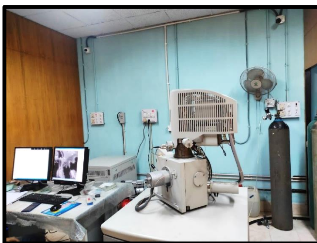
Figure 3.8: Optical image of FEI INSPECT F50 FESEM machine.
