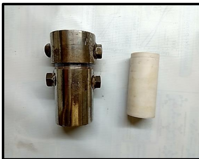
Figure 3.2: Autoclave with Teflon container.
