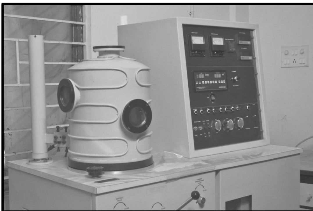
Figure 3.5: Thermal evaporator unit with accessories.
