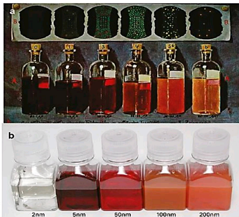
Picture 1: Size dependence of gold colloid optical properties.
