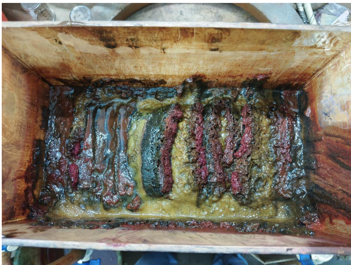
Fig. 5.10: Sludge formed during removal of Rhodamine B
