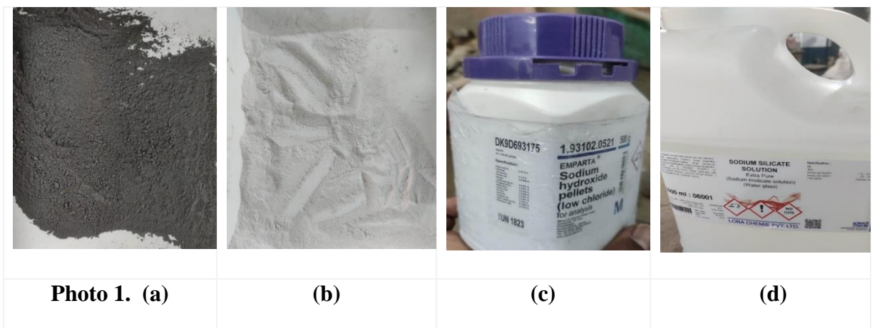
Fig. 2(a) shows dry FA, (b) shows dry GGBFS, (c) shows NaOH pellets, (d) shows \text{Na}_2\text{SiO}_3 solution
