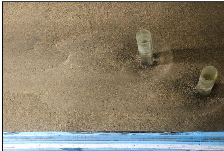
Fig 5.4 Piers placed at the working section of the flume
