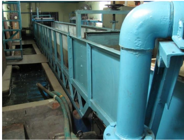
Fig 5.1 Tilting flume used during the experimentation
