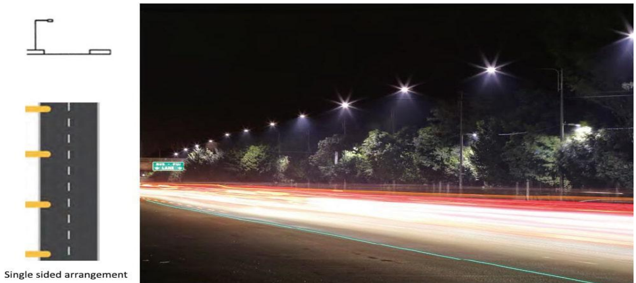
Fig 2.9. Single sided arrangement (arrangement at only one side, upper side or bottom side)
