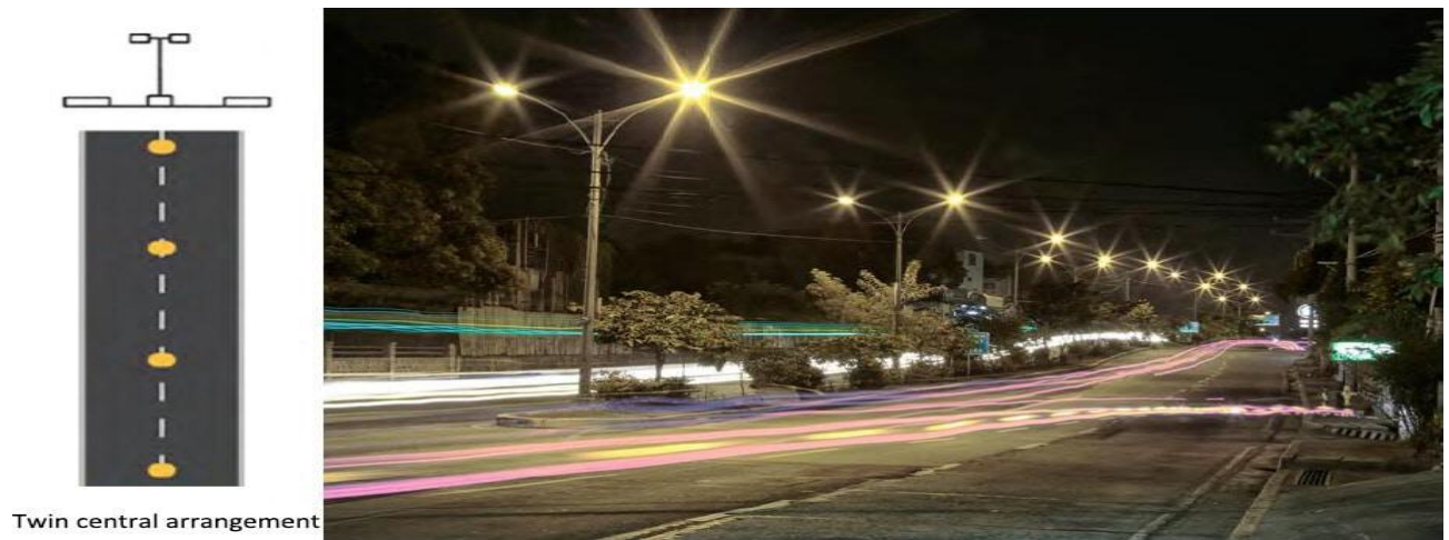
Fig 2.12. Twin central arrangement(median arrangement)
