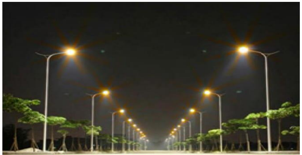
Fig 2.11. Opposite arrangement(two-sided arrangement)
