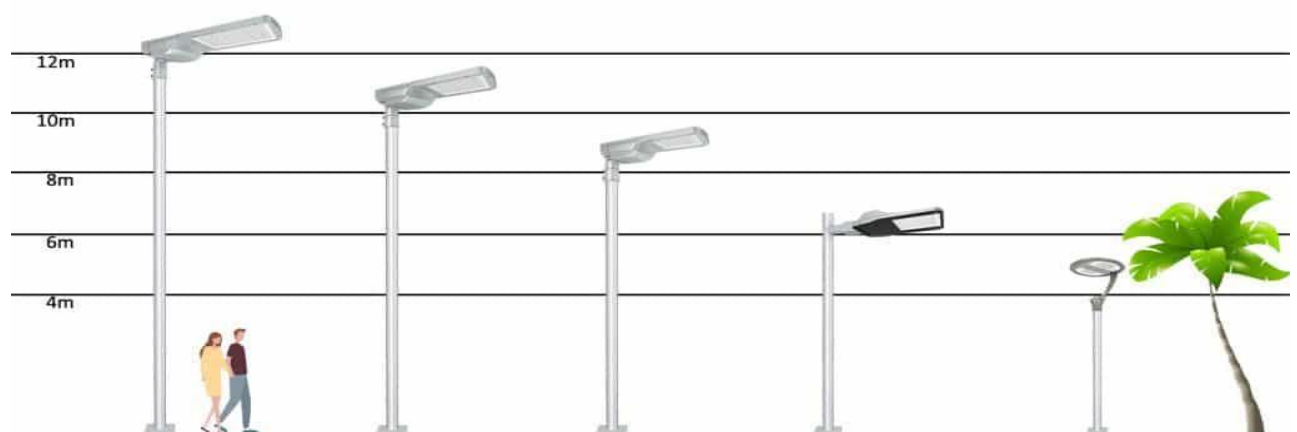
Fig 2.3. Installation height of street light luminaires
