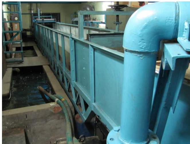
Fig 5.1 Tilting flume used during the experimentation
