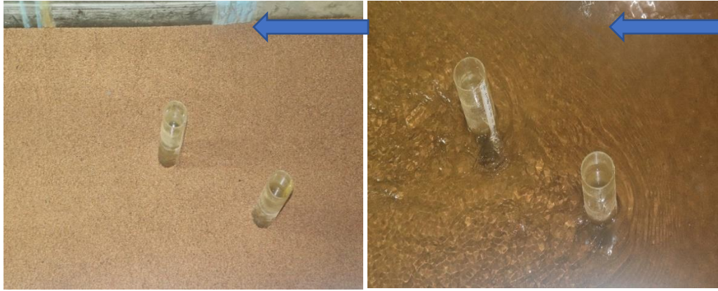
Fig 3a: Level bed, Eccentricity e = 2.5b Fig 3b: During Experiment, Eccentricity e = 2.5b
