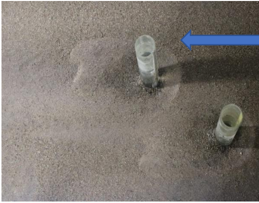
Fig 5c: Scour bed, Eccentricity e = 3b .
