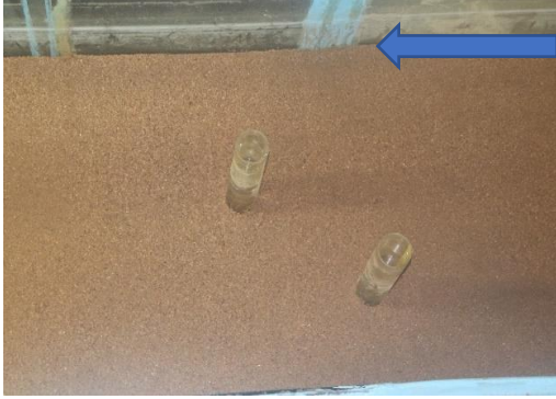
Fig 5a: Level bed, Eccentricity e = 3b
