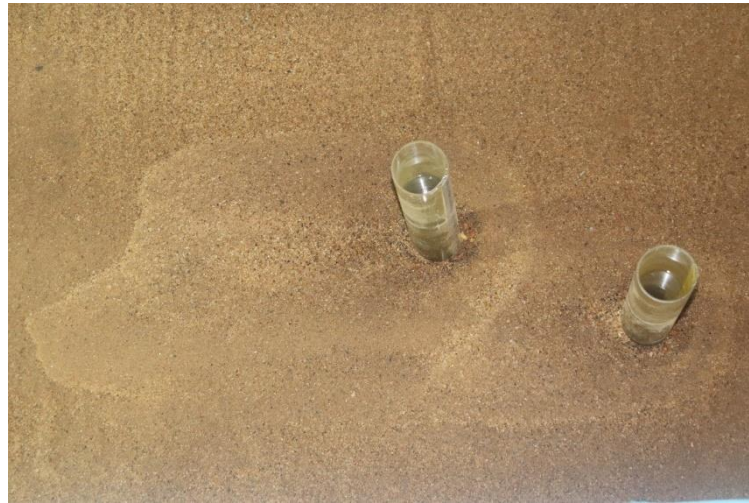
Fig.2 local scour around two eccentric piers
