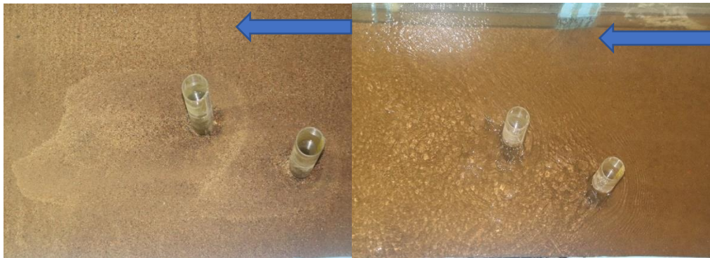
Fig 1a: Level bed, Eccentricity e = 2b
