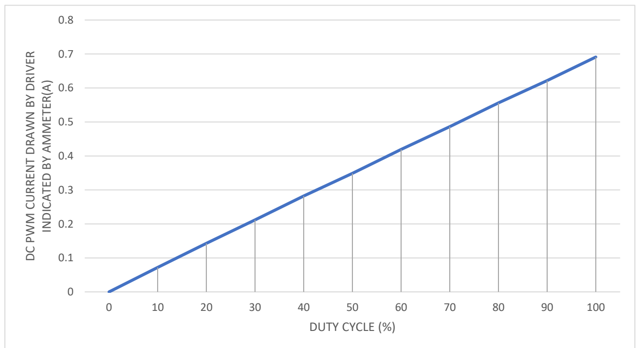
Fig 5.3 Graph showing the variations in current with respect to variations in duty cycle
