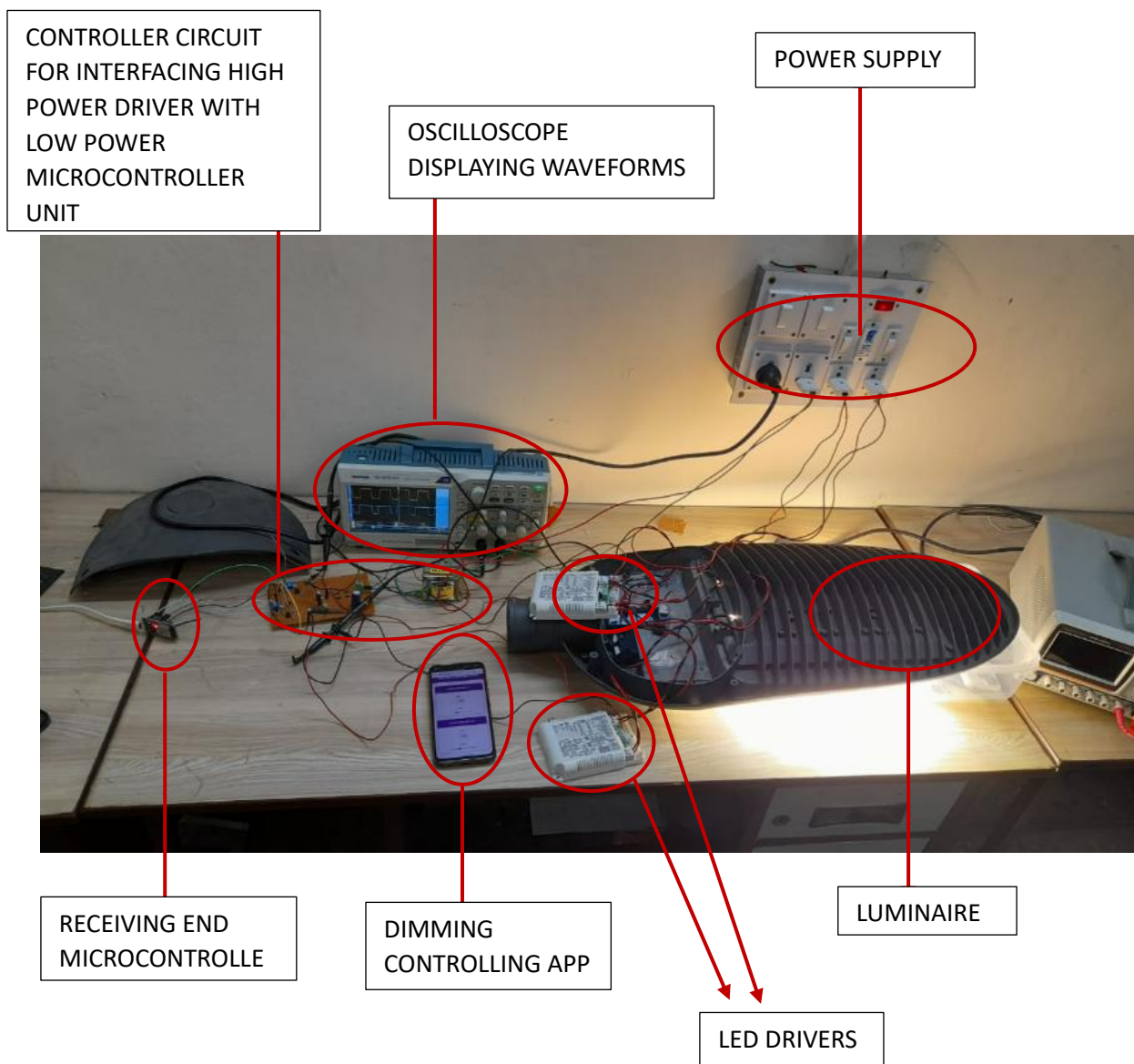
Fig 4.12 Receiving end setup showing various components used during development of the system
