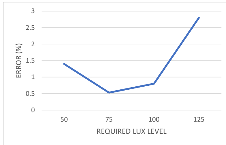
Fig 5.17 Plot showing variation of error % between required lux level and achieved lux levels with variation in required lux level
