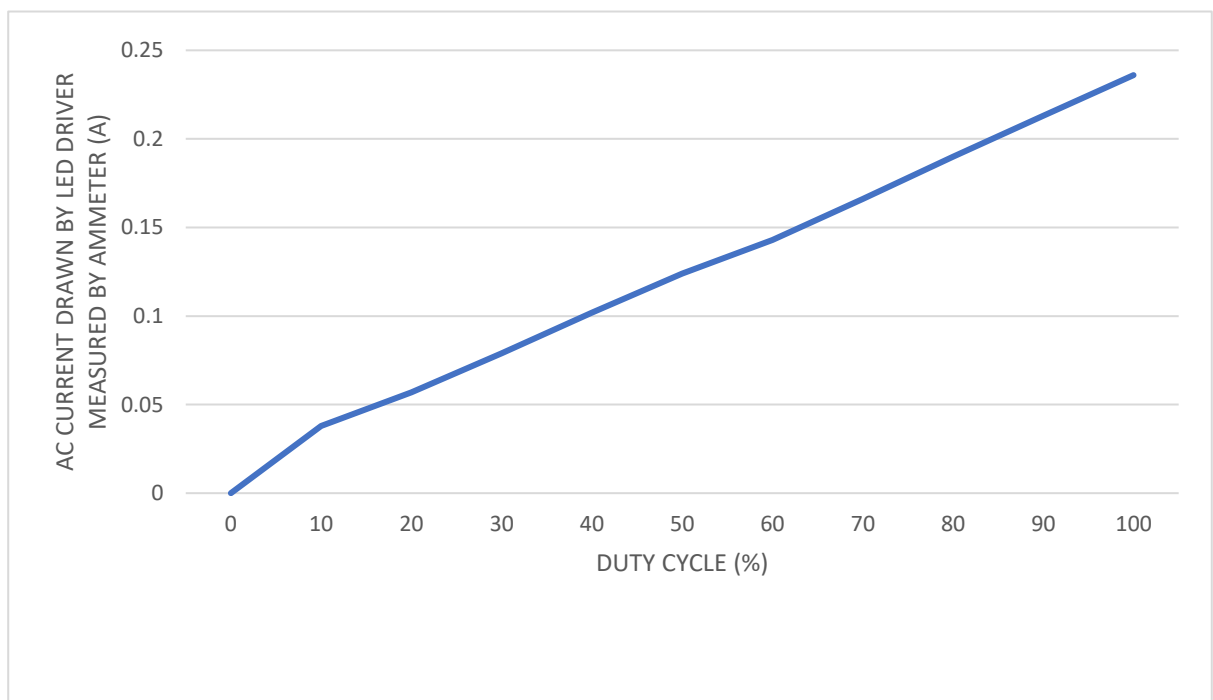
Fig 5.5 Graph showing the variations in current with respect to variations in duty cycle
