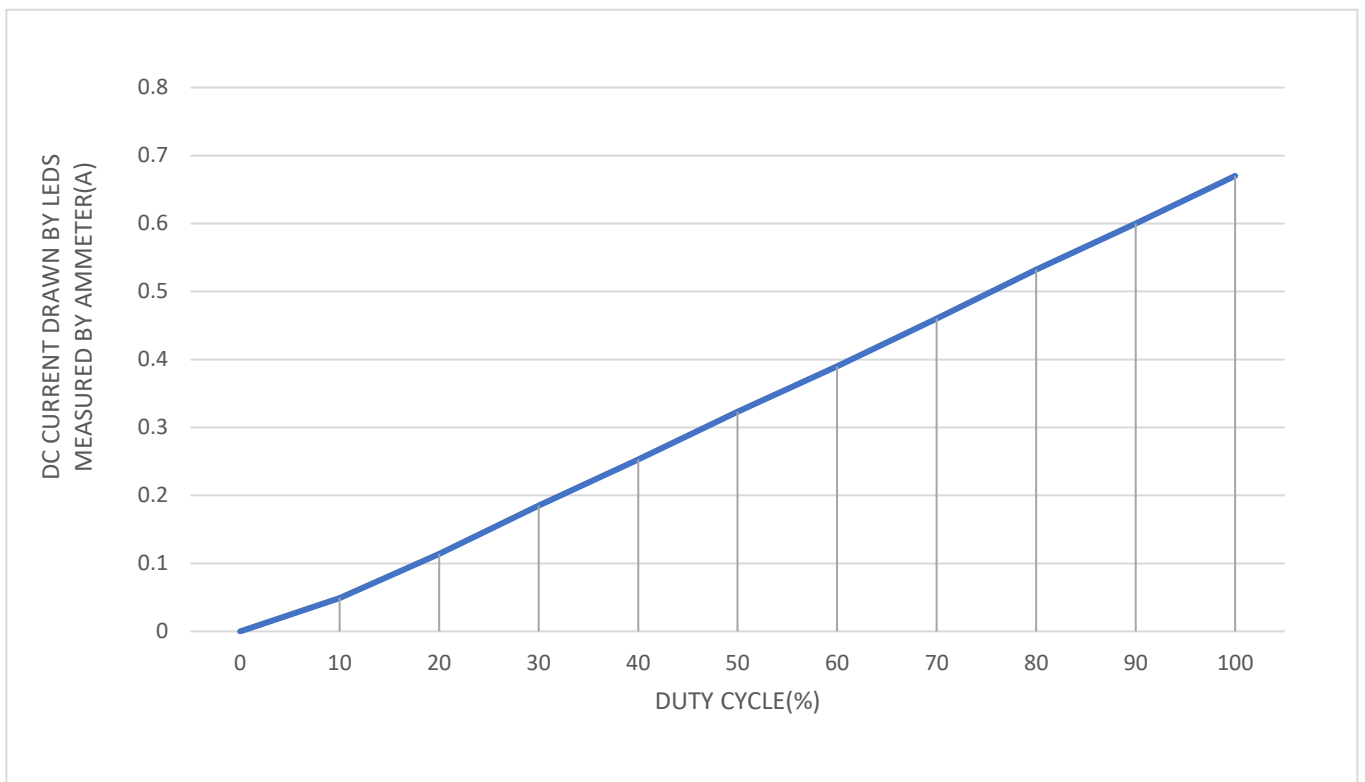
Fig 5.7 Graph showing the variations in current with respect to variations in duty cycle
