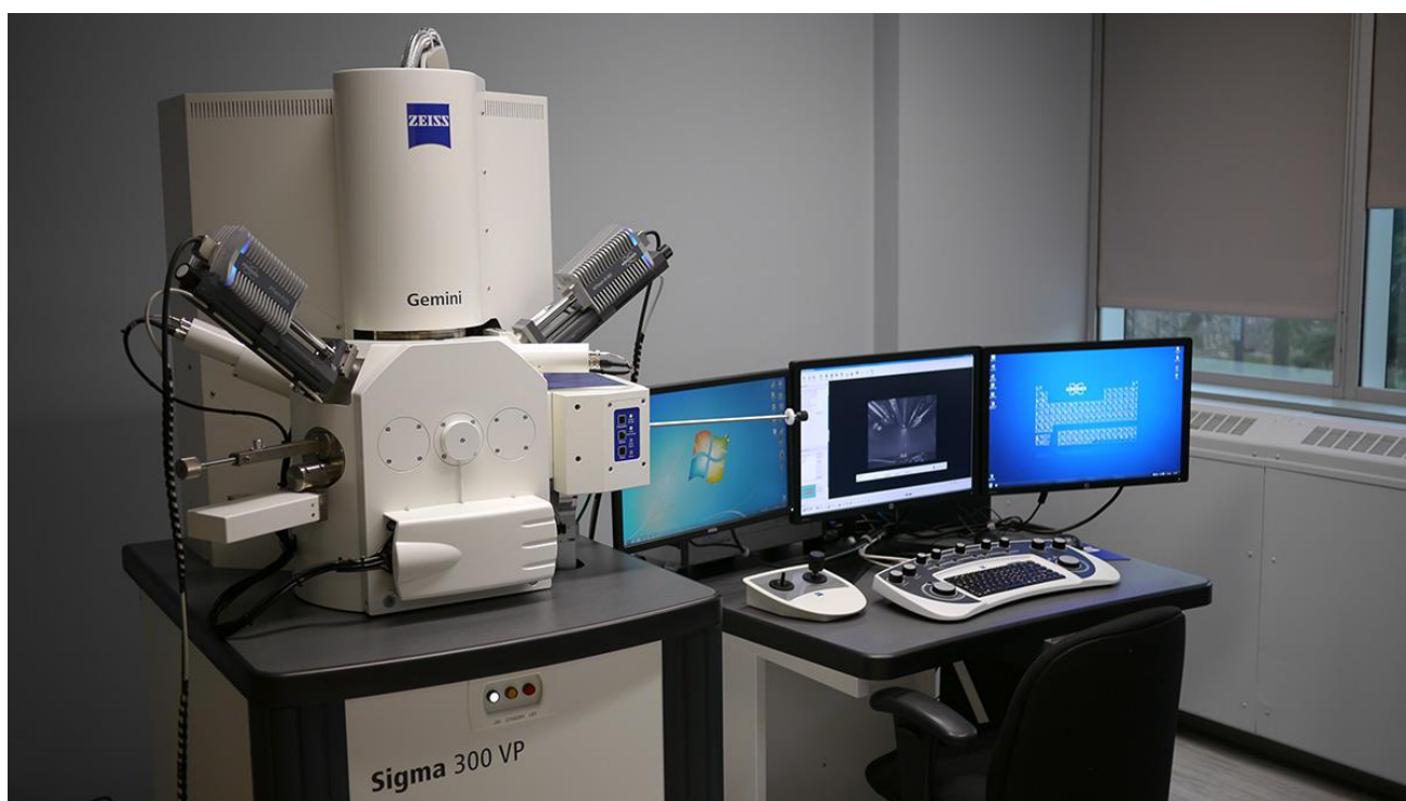
Fig 2.6- Scanning Electron Microscope (SEM) (Model-ZEISS Sigma 300 VP).
