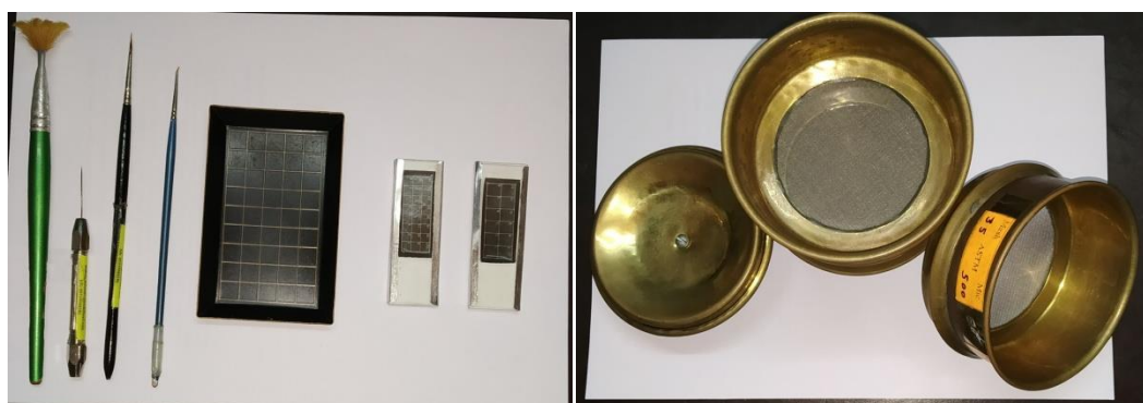
Fig 2.5- Various accessories used for picking and storing of microfossils. From left to right of the picture brushes, needle, micro paleontological tray with grids, 24 and 12 chambered slides and the sieves with a lid.
