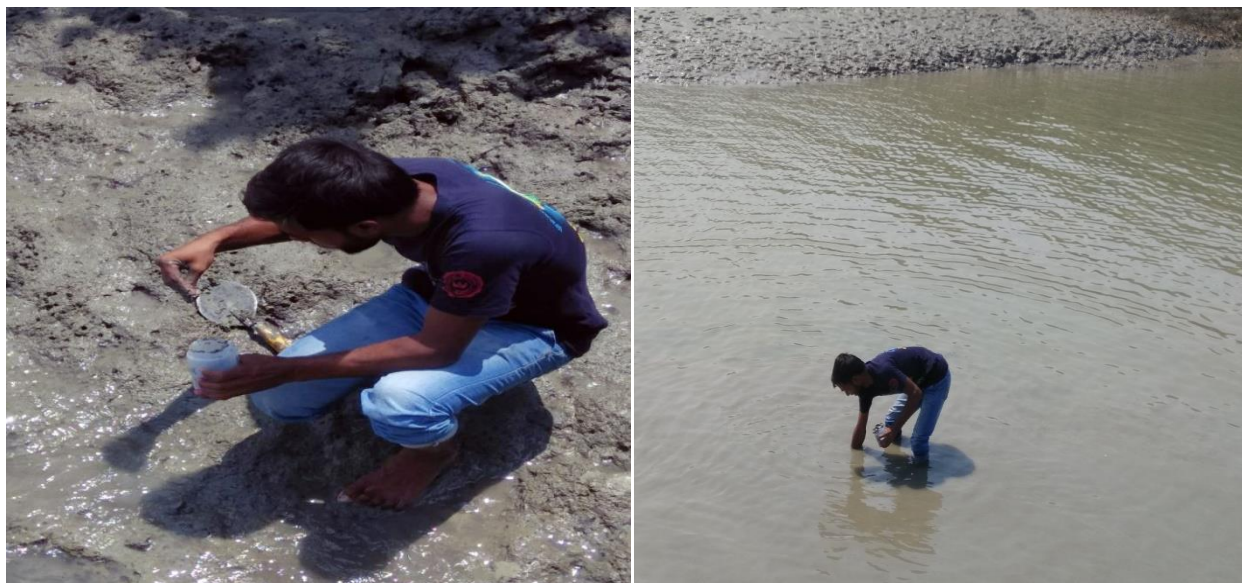
Fig.2.2- Sediment sample collection in the sampling locations.
