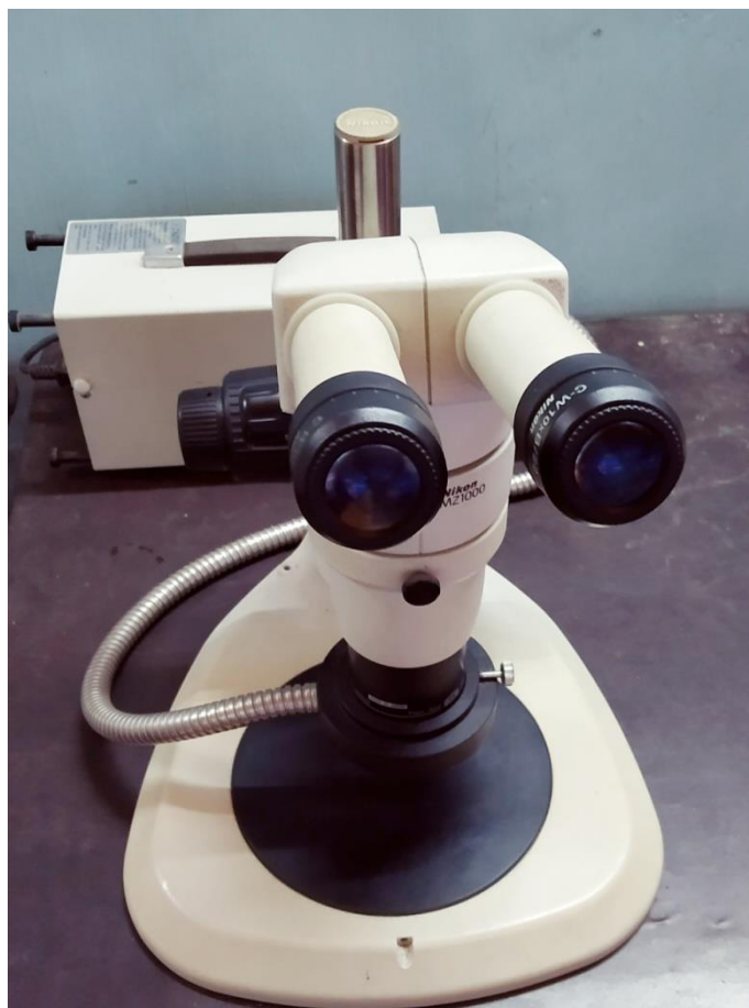
Fig.2.4- The stereozoom microscope (Nikon SMZ1000) .
