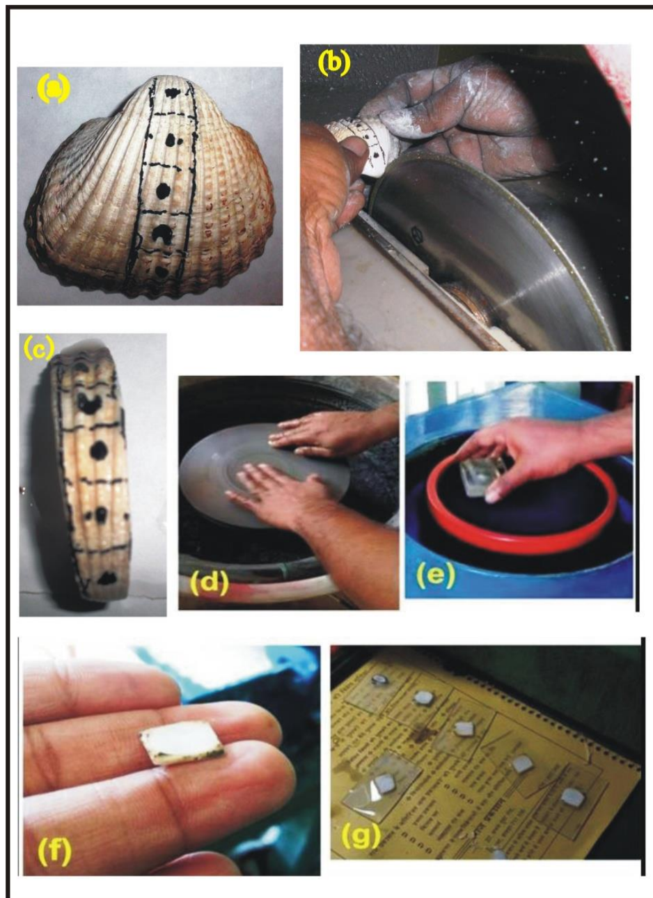
Figs 6.4(a-g) Steps those are followed to prepare a sample of 1 cm 2 for testing VH values for the species.
