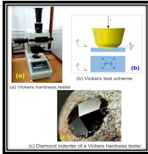
Fig 6.6 (a-c) Photographs in the laboratory during estimating VH values
