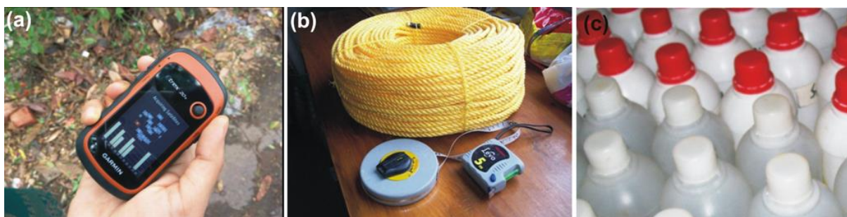
Figures 3.1(a-c) Instruments and sample bottles used during acquisition of field data and water samples, (a) Usage of GPS to detect the accurate geo-spatial coordinate of locations; (b) Ropes and tapes; (c) sample bottles for tube and dug wells
