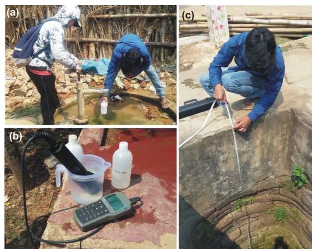
Figures 3.2 (a-c) Steps followed during sample collection, (a) Collection of water in sample bottle; (b) Estimation of some major physicochemical properties by Hanna portable multi-parameter water testing meter ; (c) In-situ field measurements of water depth
