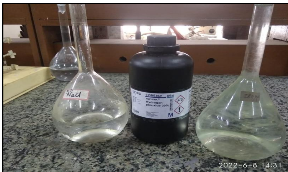
Figure 28. Natural organic material is oxidized by adding 20 mL of aqueous 0.05 M Fe (II) solution and 20 mL of hydrogen peroxide.
