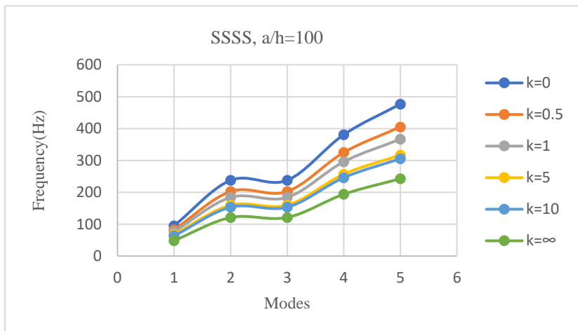
Fig 4.4.1b First five modal frequencies of Al/Al 2 O 3 FGM plate in SSSS condition for different k values and a/h=100
