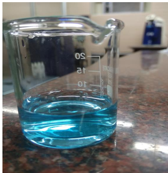
Final MB solution after 1 h 20W LED light irradiation
