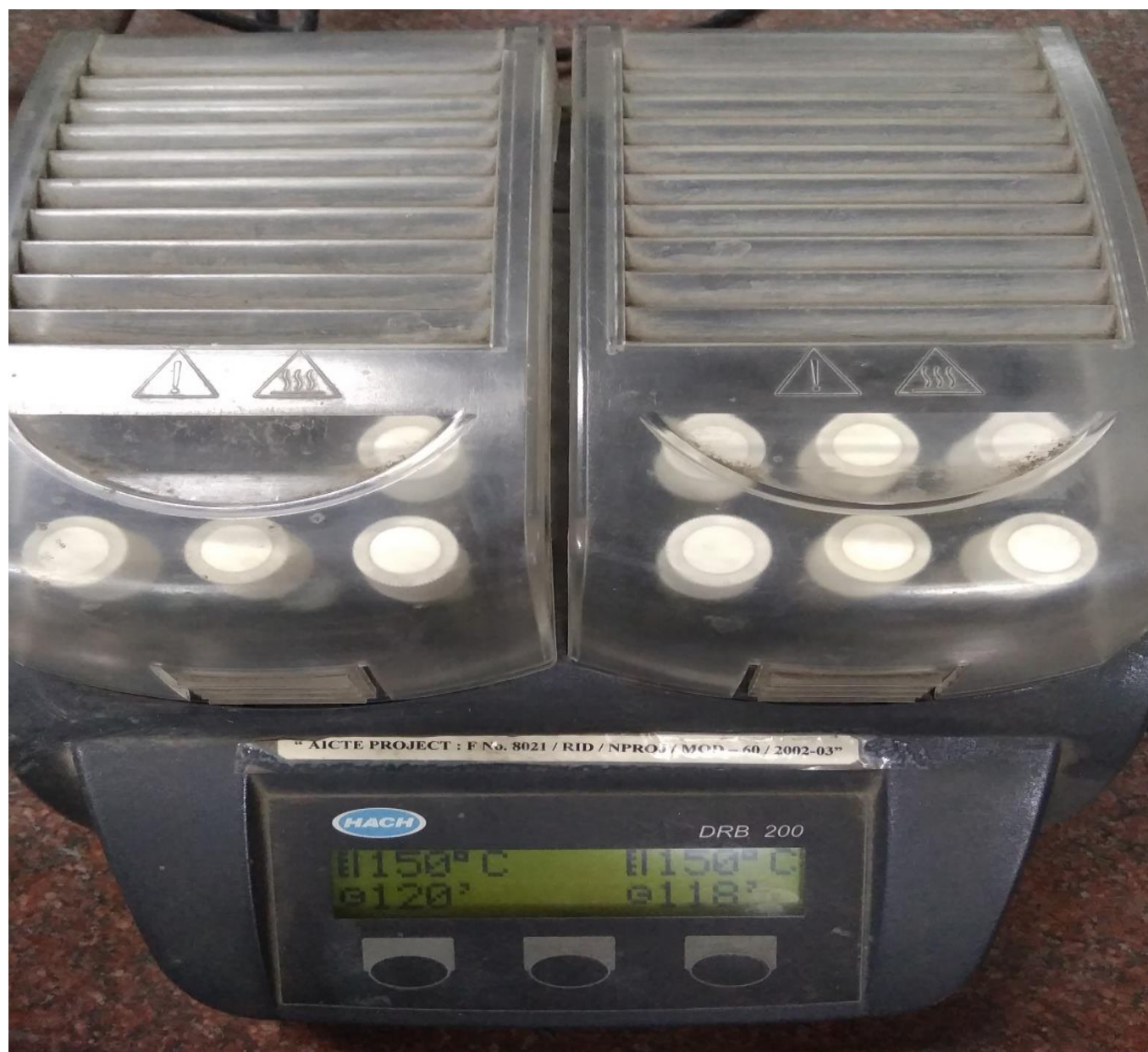
Fig 8: Closed reflux setup for determination of COD
