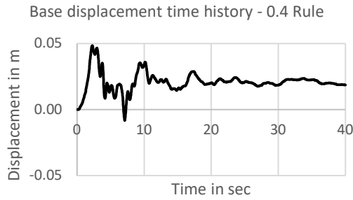
Figure 6.18 – Resultant displacement time-history for base of a G+9 regular building with pile foundation on hard soil on plane ground under Loma Prieta earthquake
