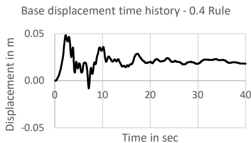
Figure 3.74 – Resultant displacement time-history for base of a G+9 regular building with isolated footing on hard soil on sloping ground under Loma Prieta earthquake
