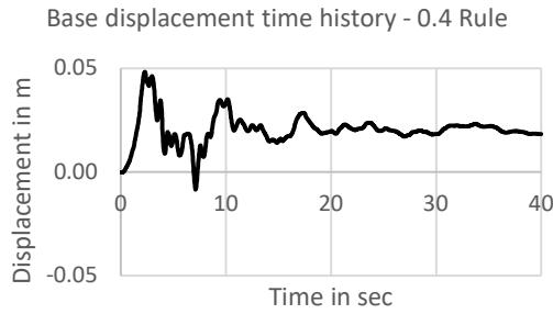
Figure 3.82 – Resultant displacement time-history for base of a G+9 vertically irregular building with isolated footing on medium soil on plane ground under Loma Prieta earthquake
