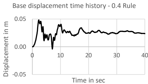
Figure 3.78 – Resultant displacement time-history for base of a G+9 regular building with isolated footing on medium soil on plane ground under Loma Prieta earthquake
