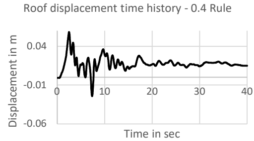
Figure 3.107 – Resultant displacement time-history for roof of a G+9 regular building with isolated footing on soft soil on sloping ground under Loma Prieta earthquake
