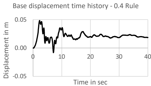
Figure 4.14 – Resultant displacement time-history for base of a G+9 regular building with isolated footing on soil 1 on sloping ground under Loma Prieta earthquake
