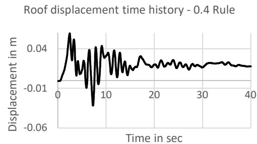
Figure 4.15 – Resultant displacement time-history for roof of a G+9 regular building with isolated footing on soil 1 on sloping ground under Loma Prieta earthquake
