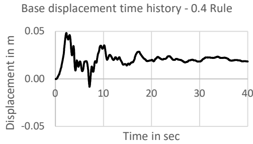
Figure 4.6 – Resultant displacement time-history for base of a G+9 vertically irregular building with isolated footing on soil 1 on plane ground under Loma Prieta earthquake
