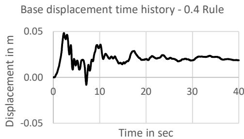
Figure 3.90 – Resultant displacement time-history for base of a G+9 regular building with isolated footing on medium soil on sloping ground under Loma Prieta earthquake
