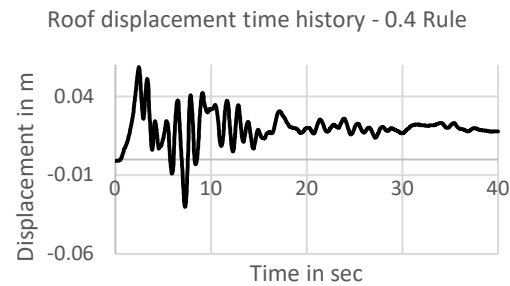
Figure 3.91 – Resultant displacement time-history for roof of a G+9 regular building with isolated footing on medium soil on sloping ground under Loma Prieta earthquake
