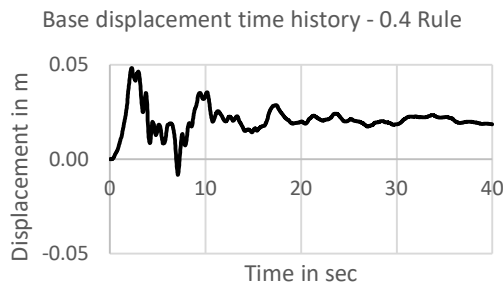
Figure 3.66 – Resultant displacement time-history for base of a G+9 vertically irregular building with isolated footing on hard soil on plane ground under Loma Prieta earthquake
