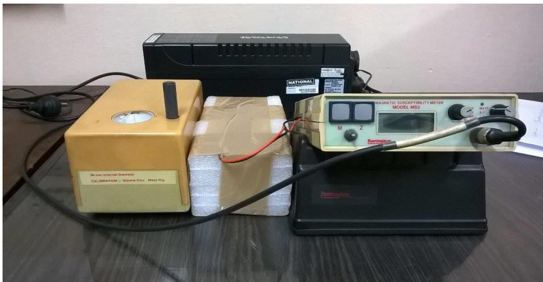
Figure 5.1. Bartington Susceptibility Meter (Model: MS2) in AMS laboratory, JU
