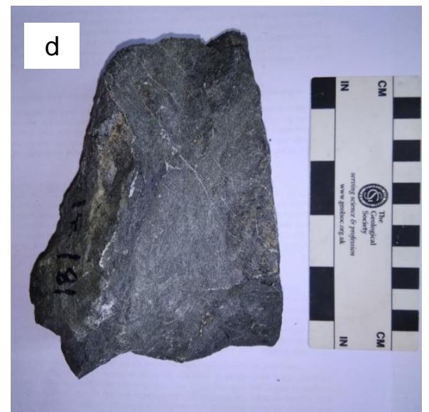
Fig 5: Representative samples of different rock types. (a) Serpentinized peridotite; (b,c) Spinifex-textured komatiites; (d) Metabasalt
