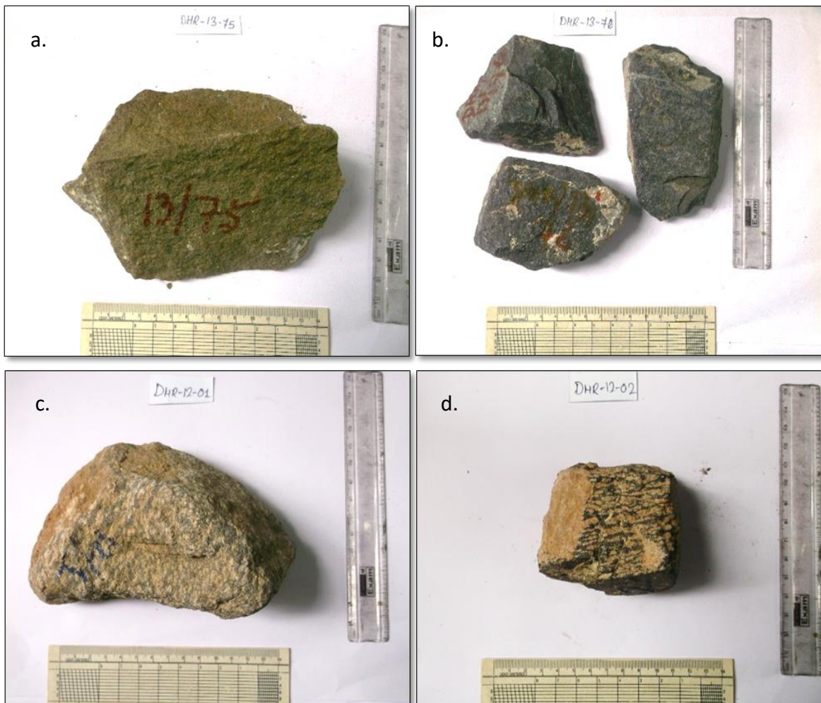
Fig 3 – Photographs of hand specimens illustrating different textures in chromite bearing rocks from Talur Magnesite Mines. a. Dunite. b. Massive chromitite. c. Schlieren banded chromitite. d. Net-textured chromitite.
