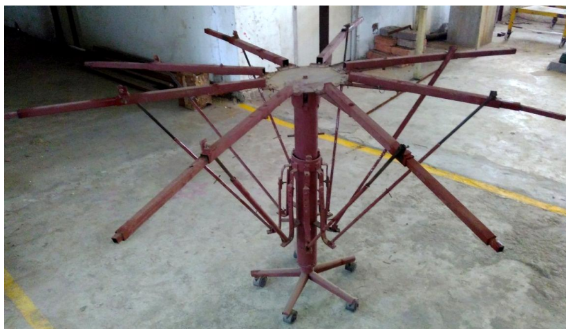
Figure 4.7 (a) Welder's job table (open)
