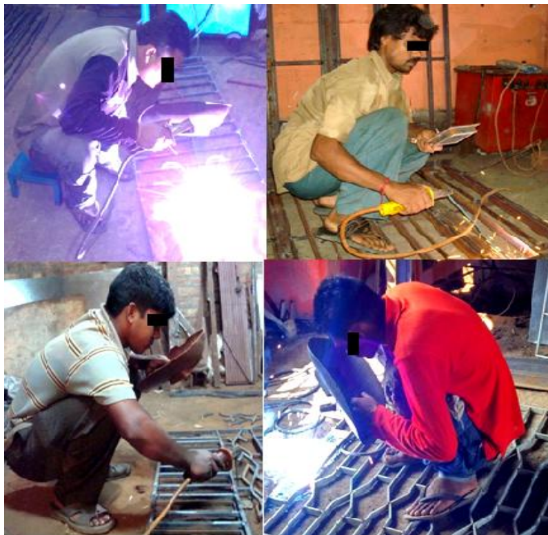
Figure 5.9 Actual working posture of welders
