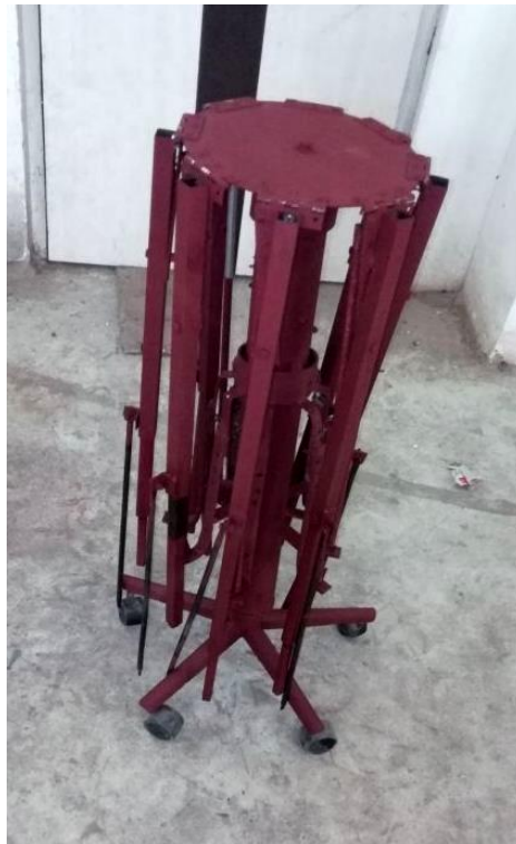
Figure 4.7 (b) Welder's job table (folded)
