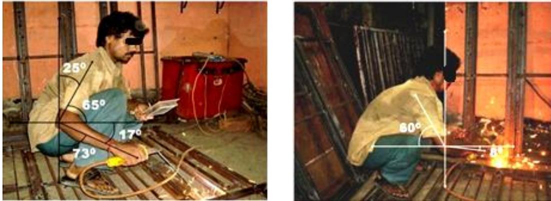
Figure 5.4 (a) Upper and lower arm angle Figure 5.4(b) Lower arm abduction angle
