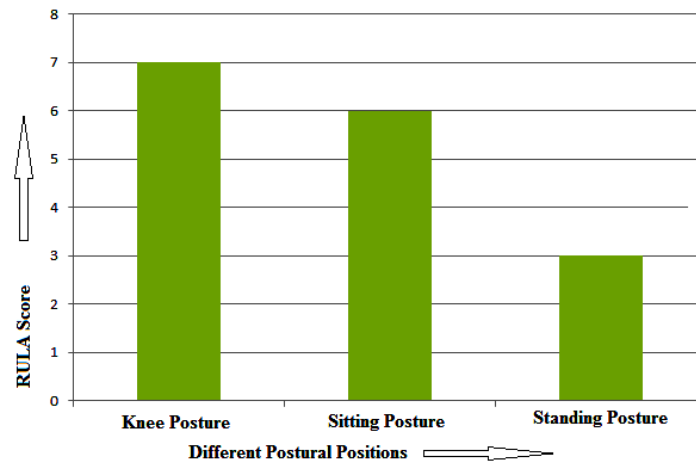
Figure 5.36 RULA score vs different postural positions of welder
