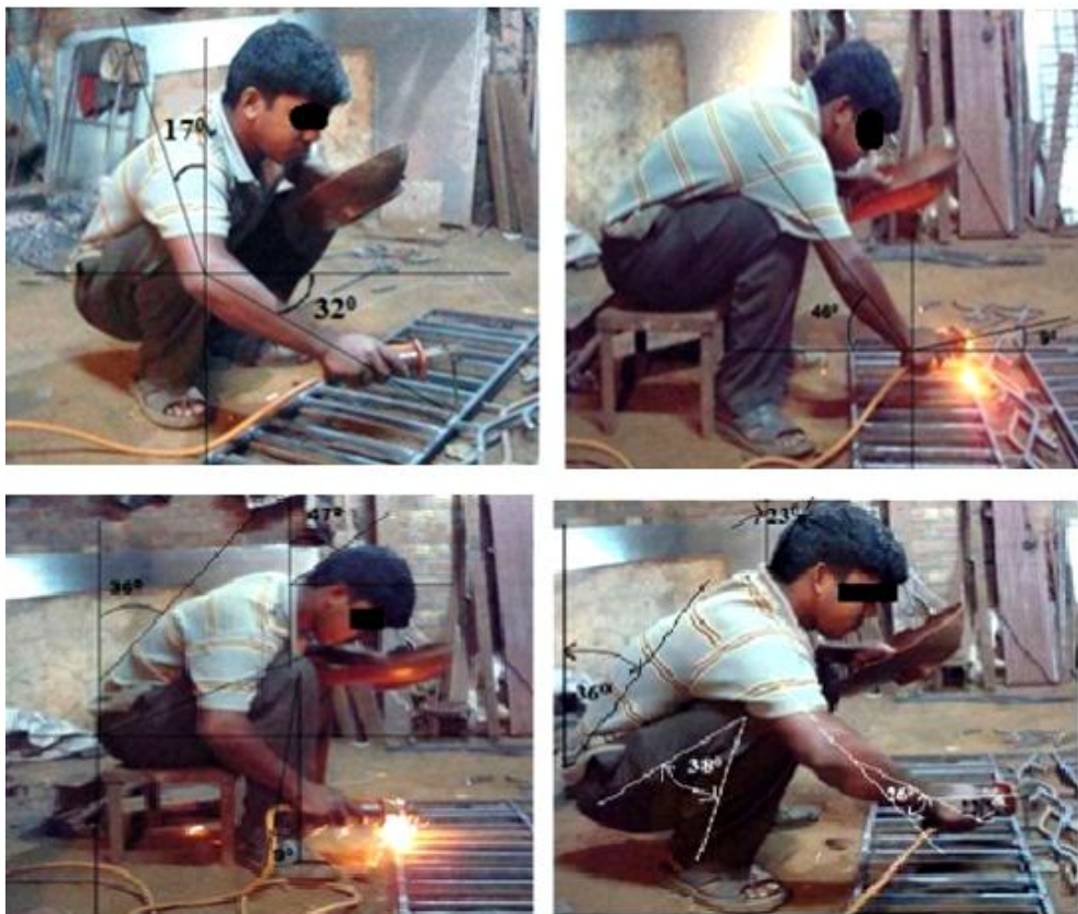
Figure 5.2 Different angular position of body parts of welder
