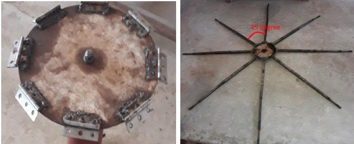
Figure 4.4 (a) MS base plate (top view) Figure 4.4 (b) MS base plate with square pipe
