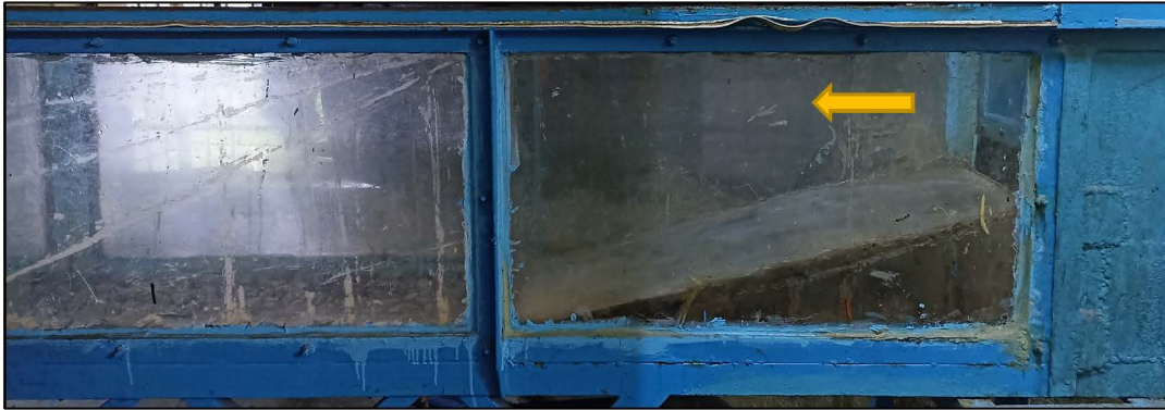
Fig. 6.6. Ramp fitted at the inlet for jump development.
