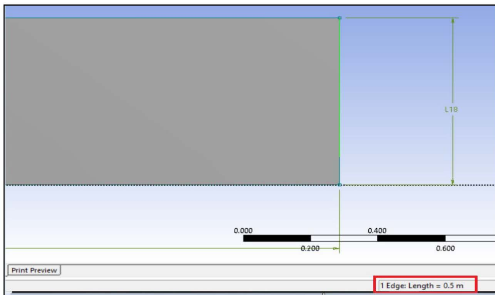
Fig. 4.4. Upper portion of tailgate shown in green and its dimensions enclosed in red box.
