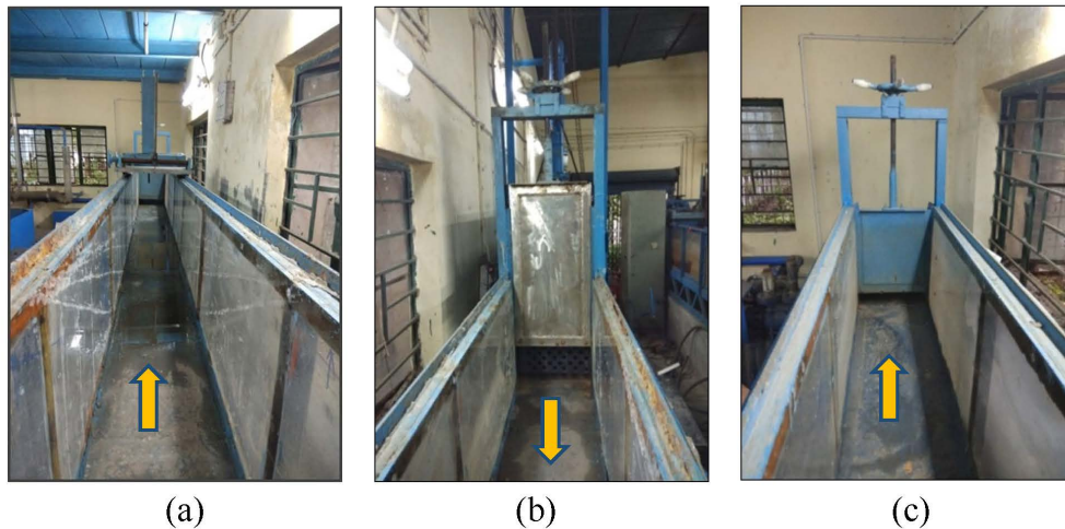
Fig. 5.3. Experimental flume (a) Flume bed, (b) Inlet gate, and (c) Outlet gate.
