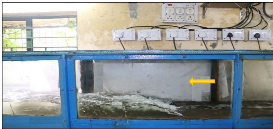
Fig. 3.7. H-jump formation during experimentation in the laboratory.
