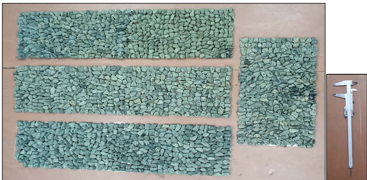
Fig. 6.3. Preparation of the arrangement with gravel bed materials.
