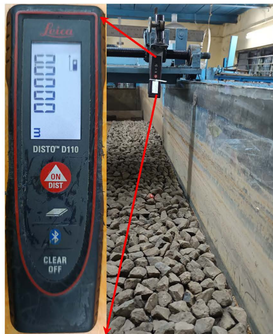
Fig. 6.5. Roughness height measurement using laser distance sensor.
