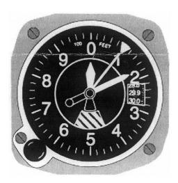
Diagram showing the face of the "three-pointer" sensitive aircraft altimeter displaying an altitude. Calculate the altitude of the aircraft.
