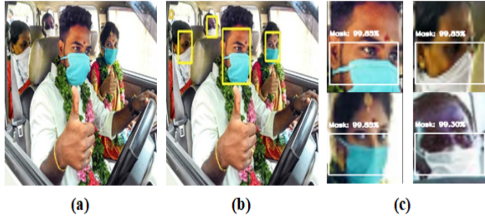
Figure 5.13: Testing flow: a) Input image. b) Face detected image. c) Mask detected images with confidence level
