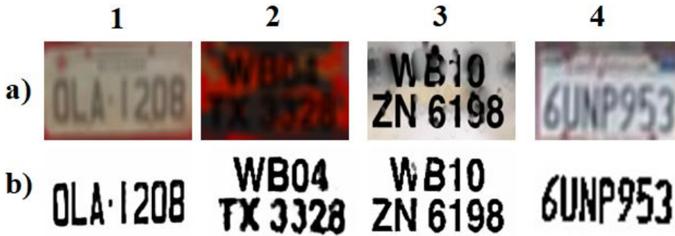
Figure 4.7: Sample images and ground truth produced by the proposed algorithm with different environment condition: 1) blur. 2) Tricky background patch and distortion. 3) Water bubble effect. 4) Extra lighting condition.
