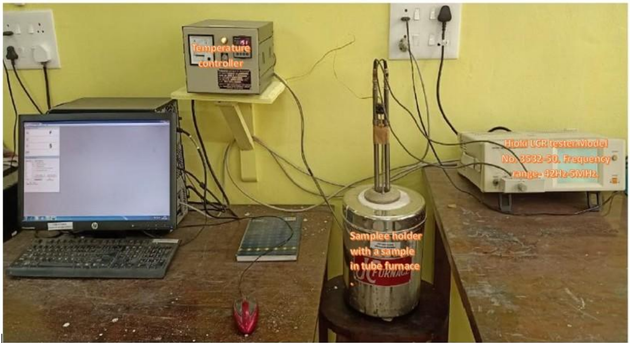
Fig. 3.5: Experimental set-up for electrical measurements
