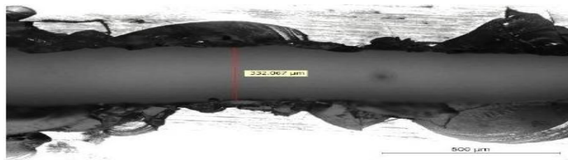
Fig. 5.45 Cross section of micro-slot of 1.35mm machining depth cut at 55V/200Hz/NaOH30wt%/40%/40mm IEG
