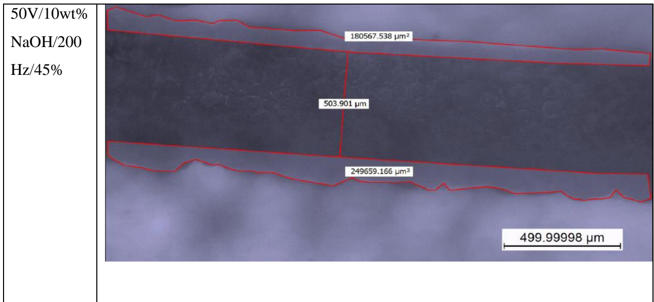
Fig.5.4 Optical microscopic images of micro-channel with HAZ area at different conditions
