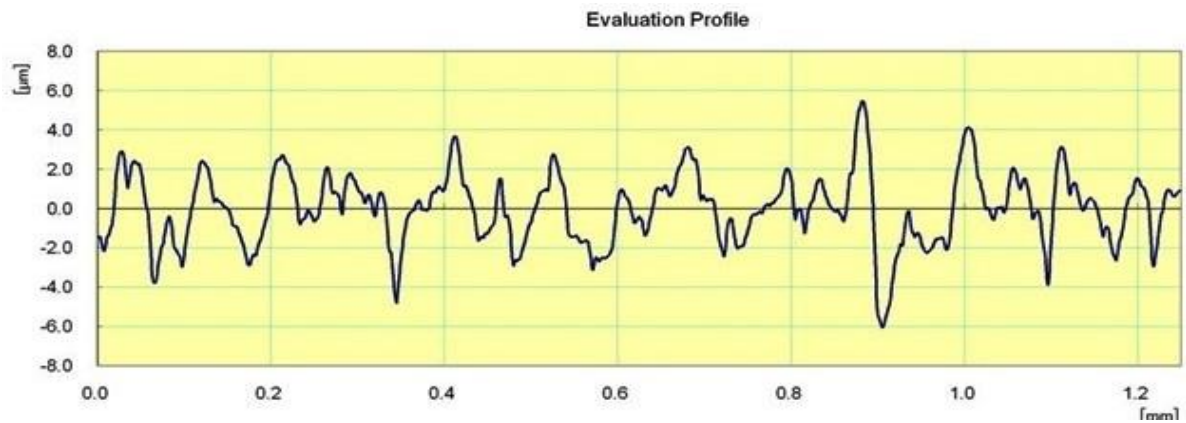
Fig. 5.12 Surface texture of micro-channel at 50V/25wt% NaOH:KOH:: 1:0/55%/600Hz
