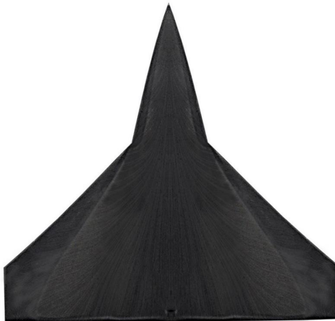
Figure 5.1(b) Oil Flow visualisation at 5^\circ AoA
