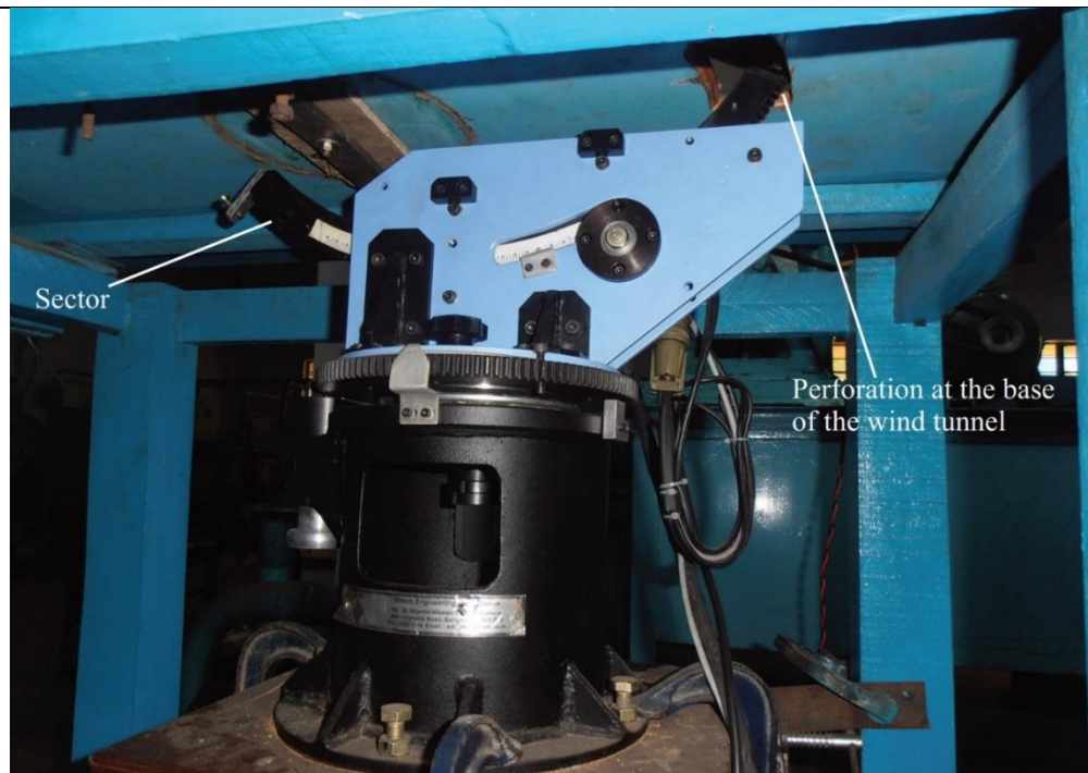
Plate 3.2 Photograph of wing traversing mechanism
