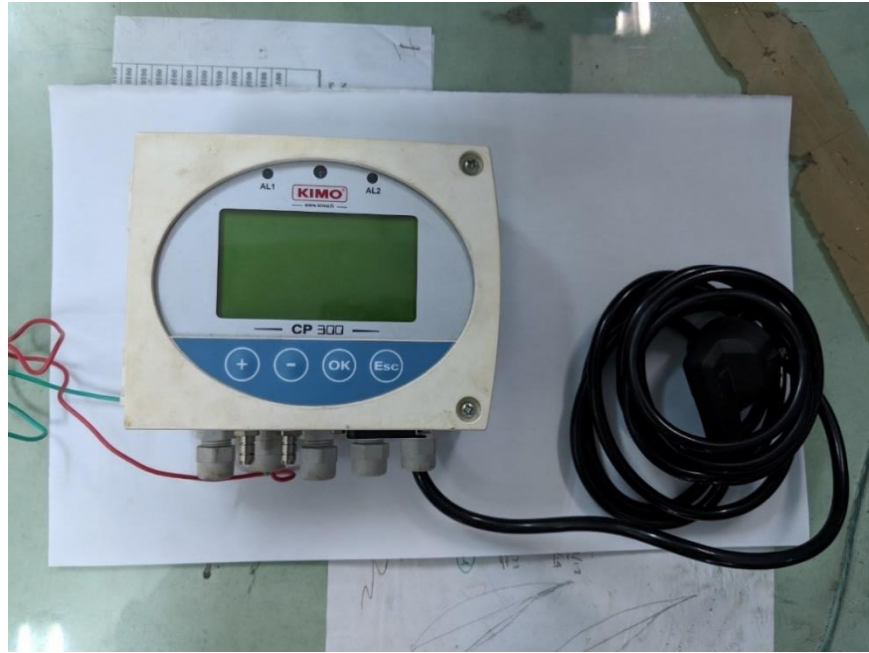
Plate 3.9 Photograph of differential pressure transducer
