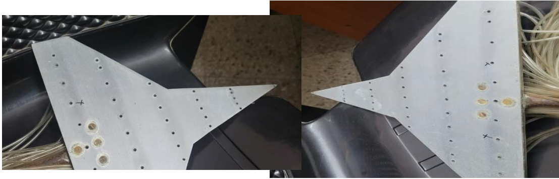
Plate 3.10 Surface pressure measurement station of wing
