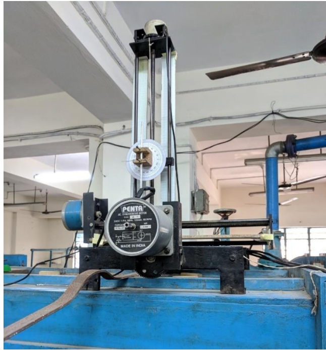
Plate 3.3 Photograph of probe traversing mechanism
