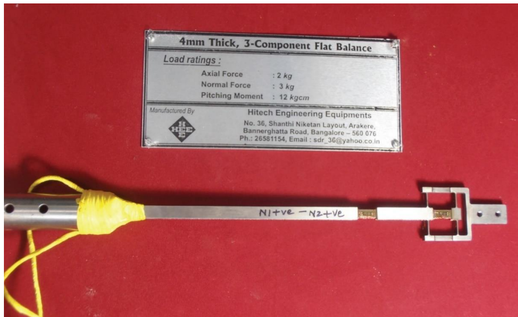
Plate 3.4 Photograph of 3-component strain gage balance
