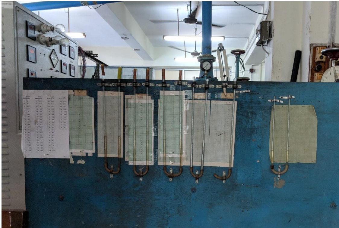
Plate 3.8 Photograph of array of U-tube manometer during 3-hole probe calibration
