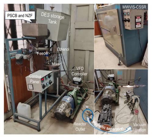
**Figure 5. 20.** Experimental setup of (a) screw feeder, mixer, diaphragm pump and VFD controller (b) MWVIS-CSSR (c) vacuum filtration unit
