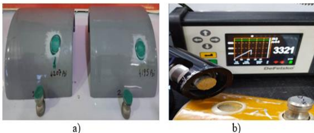
Figure 6B.30: Pull-off Adhesion Tested Samples (before HWI Test) - a) LE, b) PU
