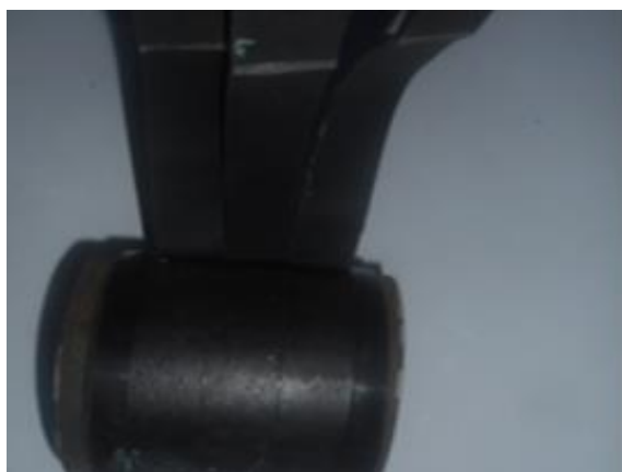
Peel strength tested 3p/2p CAT coated pipe sample after hot water immersion
