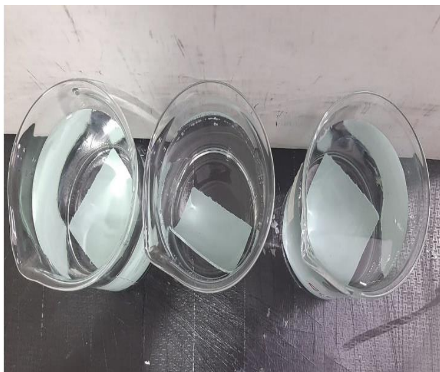
Water absorption test of VE coatings
