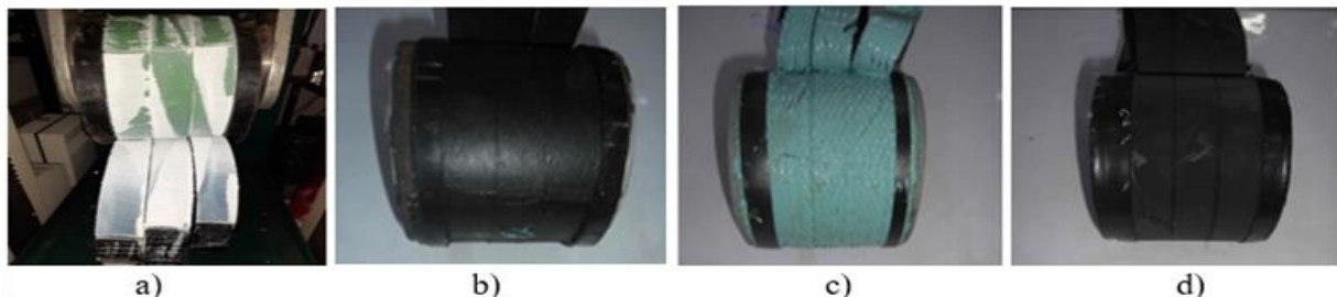
Figure 6B.29: Peel Tested Samples - a) 3LPE, b) 3p/2p CAT, c) VE, d) HSS
