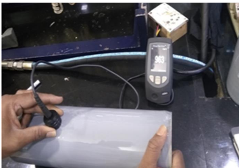
Thickness measurement on LE coated pipe sample
