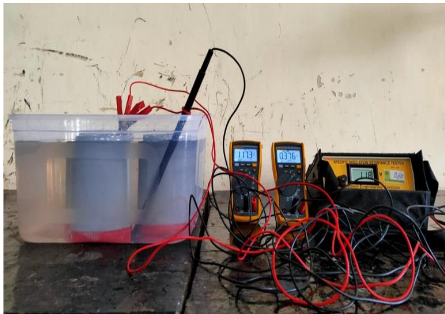
Experimental set-up for specific electrical insulation resistance test on coated pipe samples
