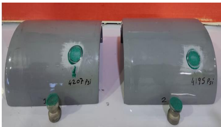
Pull-off adhesion tested LE coated pipe sample before hot water immersion
