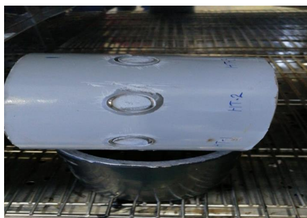
PU coated pipe sample after pull-off adhesion test at 55±5°C
