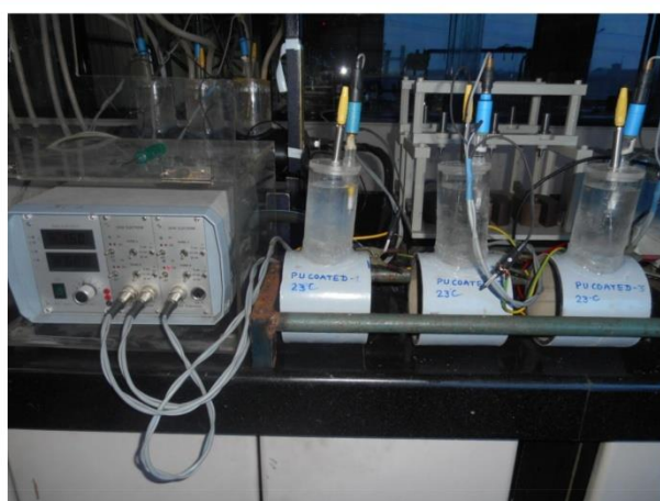
Figure 5.12: Cathodic Disbondment Test Assembly
