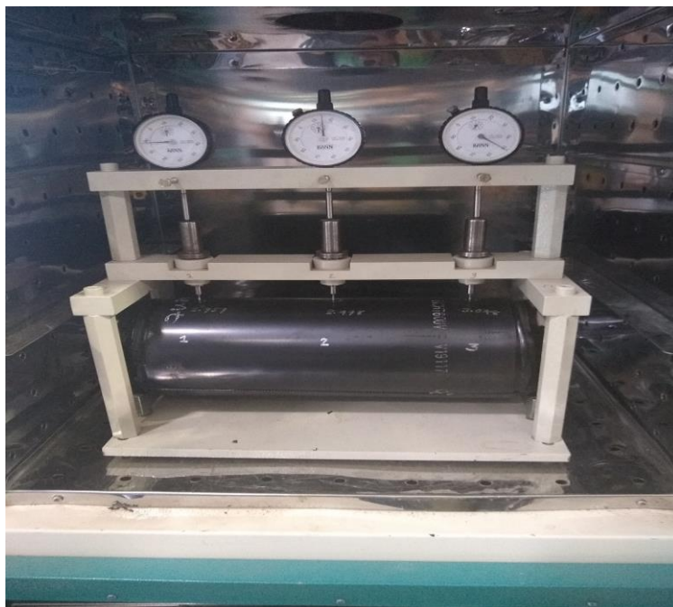
Indentation resistance test set-up for HSS coated pipe sample
