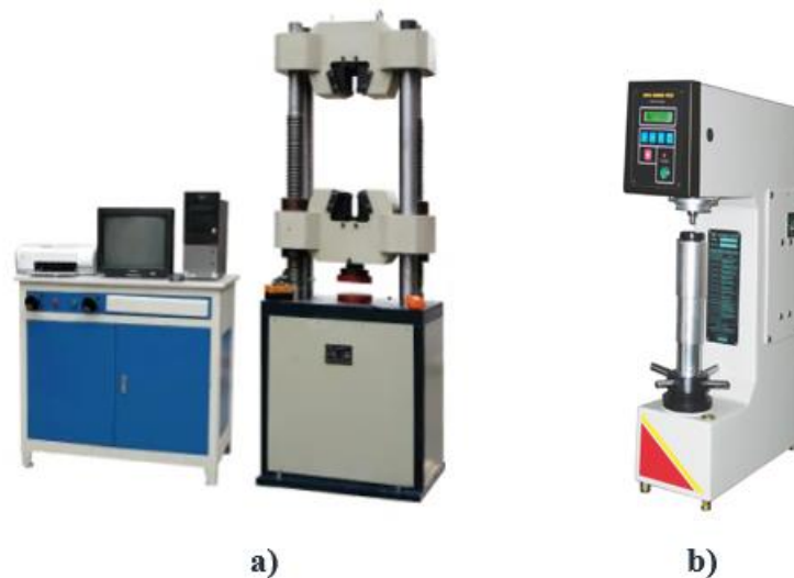
Figure 5.2: a) UTS Machine, b) Rockwell Hardness Tester
