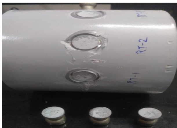
PU coated pipe sample after pull-off adhesion test at 23°C
