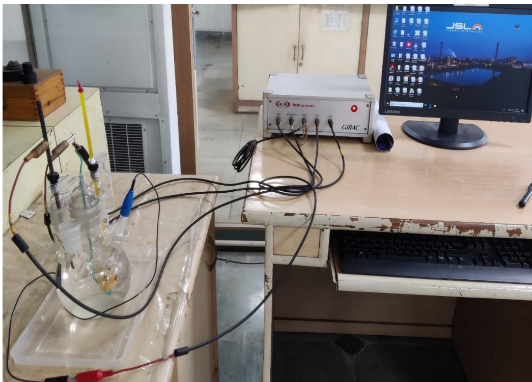
Experimental set-up for cyclic potentiodynamic polarization test (3-electrode system)
