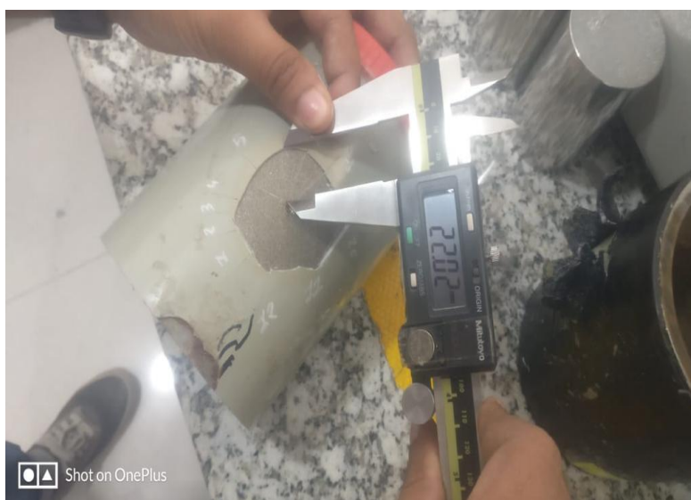
CD measurement of LE coated pipe sample
