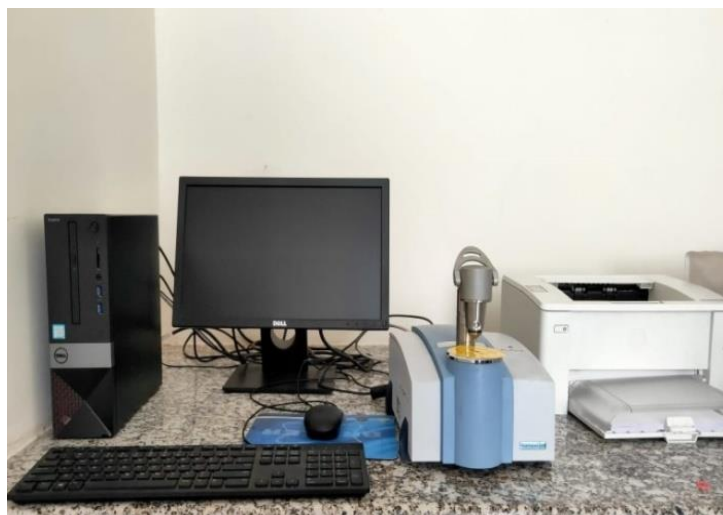
Figure 5.19: FTIR Bruker Model No. ALPHA II
