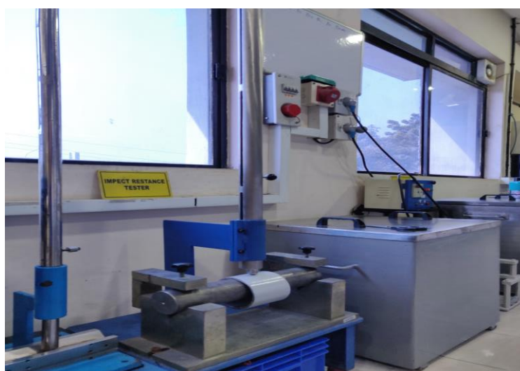
Impact resistance test on PU coated pipe sample
