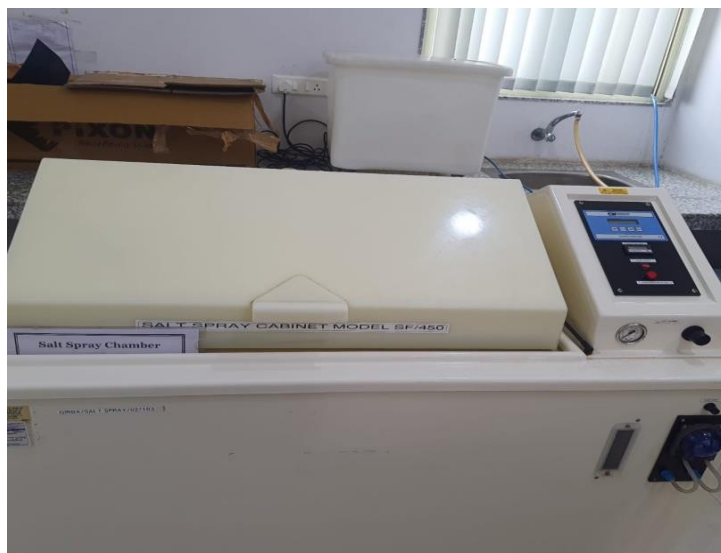
Figure 5.21: Salt Spray Chamber Model No. SF/450
