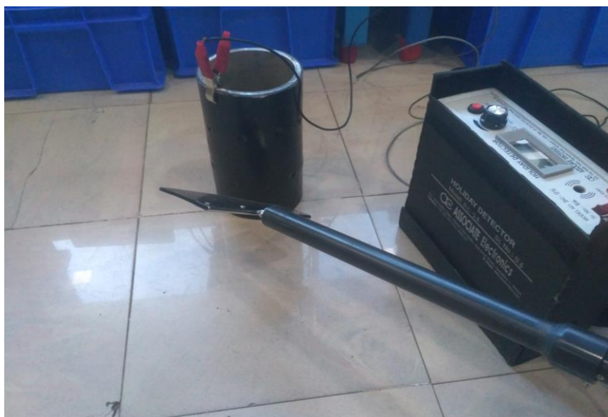
Holiday detection on 3LPE coated pipe sample
