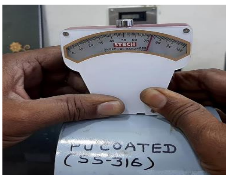
Shore D hardness measurement on PU coated pipe sample
