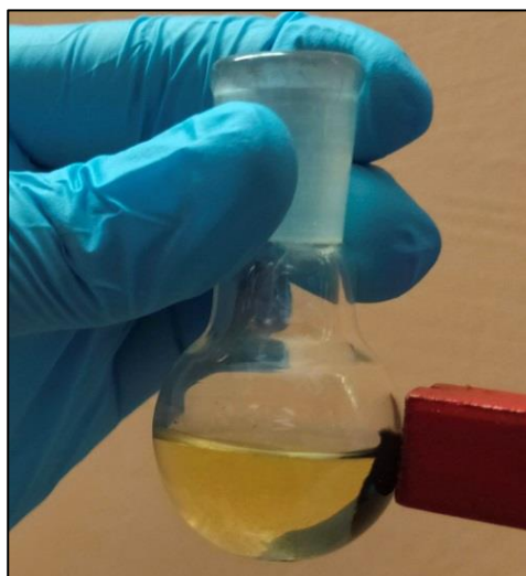
Figure-1.4 Magnetic separation of \text{Fe}_3\text{O}_4 -starch-Pd(II) catalyst by an external magnet.
