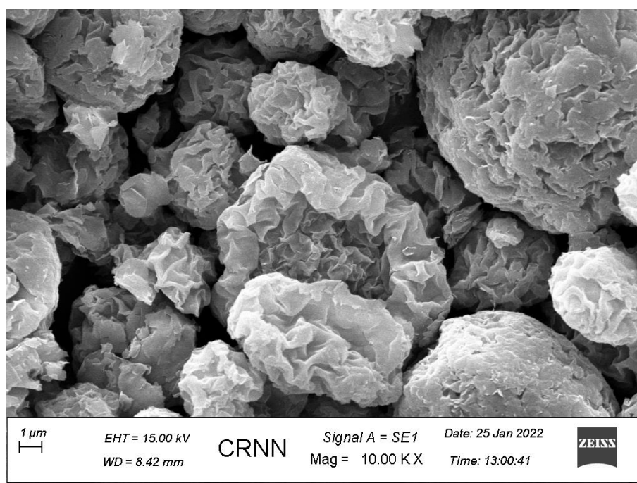
Fig 5B.17. SEM image of pure Na-MMT
