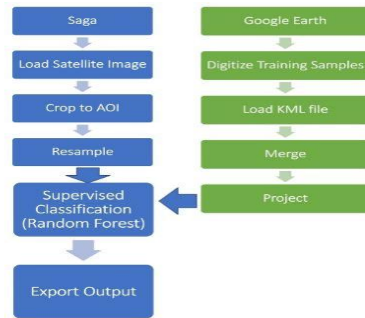
Figure 3.10. The workflow to classify LCZ as per the WUDAPT method
