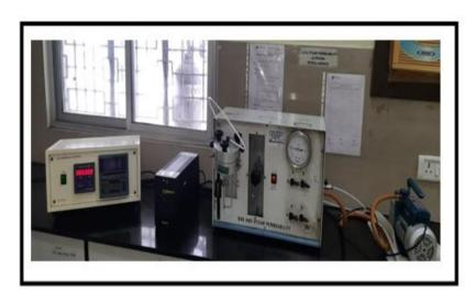
Fig-3.15: The photograph of the OTR instrument (At the Indian Institute of Packaging, Kolkata, India) used in the Barrier property determination.
