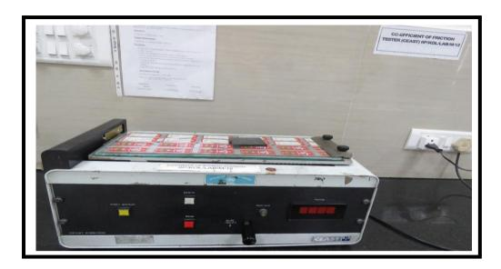
Fig-3.7: The photograph of the Coefficient of Friction testing instrument (At the Indian Institute of Packaging, Kolkata) used in the measurement of surface roughness.
