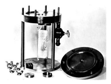
Fig-3.16: The photograph of the Manometric Gas Transmission Cell which operates within an OTR machine.
