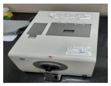
Fig-3.17: The photograph of the Konica Minolta Spectrophotometer (At the Indian Institute of Packaging, Kolkata, India).
