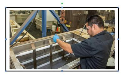
Fig-2.4: Solvent cleaning technique being applied in the industry
