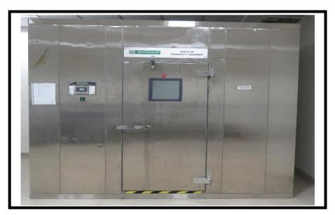
Fig-3.18: The photograph of the Humidity Chamber (At the Indian Institute of Packaging, Kolkata, India) used in the Ageing Test.
