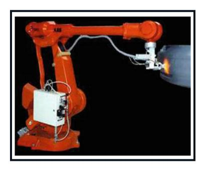
Fig-1.9: Image of flame treatment attached to robot courtesy of FTS Technologies
